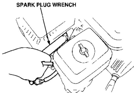
3. Inspect the spark plug. Replace it if the electrodes are worn, or if the insulator is cracked or chipped.
