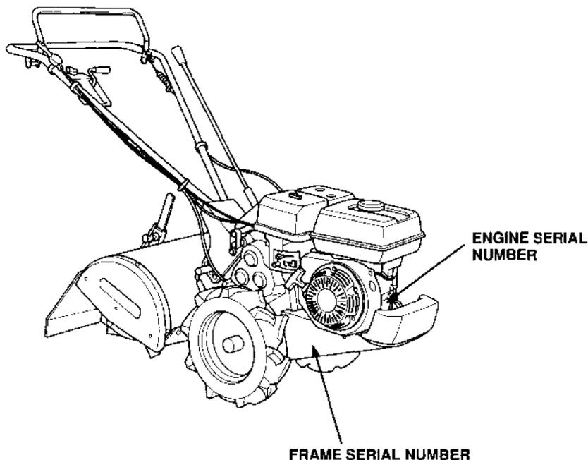
Record the engine and frame serial numbers in the spaces below. You will need this serial number when ordering parts, and when making technical or warranty inquiries (see page 64).
