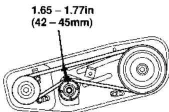
2. To adjust, loosen the four engine mounting bolts and the belt stopper attaching two bolts (front side) and move the engine forward or backward to get proper tension on the belt.
