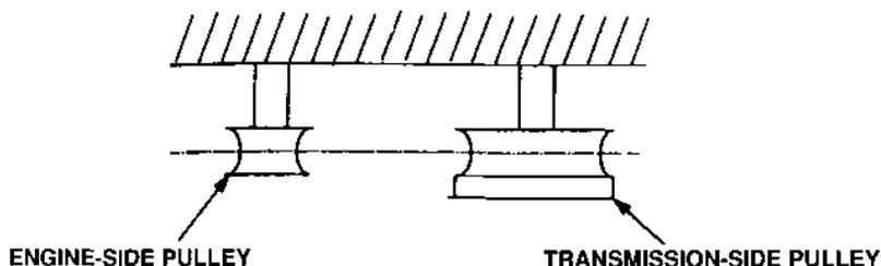
3. Loosen the belt stopper attaching bolts. Adjust the clearance between the belt stopper and the belt as illustrated with the clutch lever squeezed.
