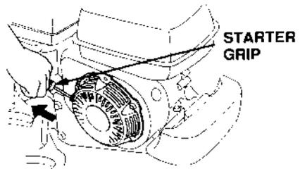
Do not allow the starter grip to snap back against the engine. Return it gently to prevent damage to the starter.
