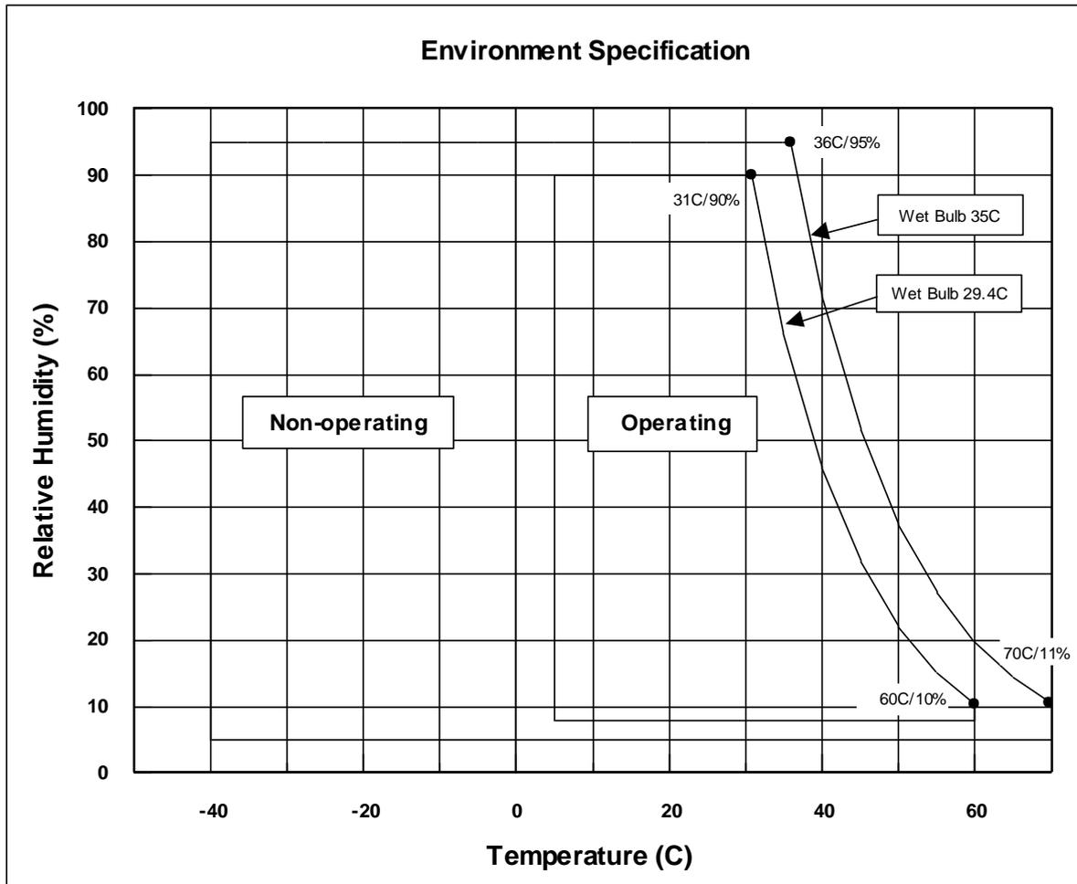
Figure 4 Limits of temperature and humidity
