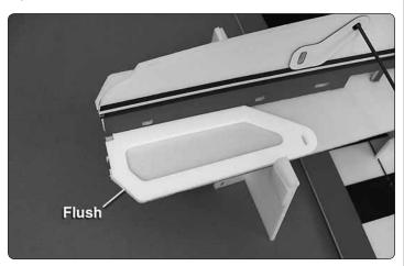
☐ 3. Glue the two **horizontal fuselage doublers** to the front of the fuselage. Make sure they are flush with the front of the fuselage and against the vertical fuselage.
