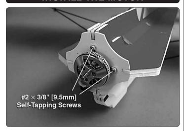
1. Install the motor to the motor mount using the included #2 x 3/8" [9.5mm] self-tapping screws.
