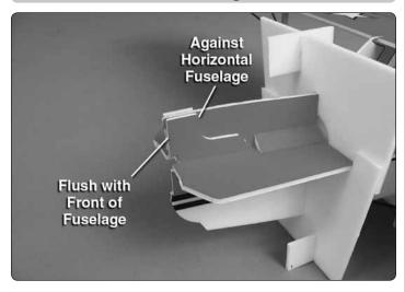
☐ 1. Remove the motor mount and glue the **upper motor doubler** to the front of the vertical fuselage. The front of the upper motor doubler should be flush with the front of the fuselage.
