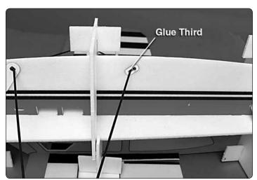
■ 8. Position the medium brace doublers so that both carbon rods pass through the brace doubler. Glue the brace doubler and carbon rod to the vertical fuselage.
