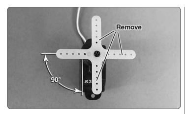
☑ 2. Connect the elevator servo to your receiver. Remove the servo screw from the servo and install a large servo arm onto the servo. Center the trims on the transmitter. Position the servo arm so that one arm is perpendicular to the centerline of the servo as shown. Use diagonal pliers to remove the three extra servo arms.
