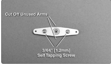
☐ 3. Attach the servo arm extension to the servo arm using two 3/64" [1.2mm] self tapping screws.
