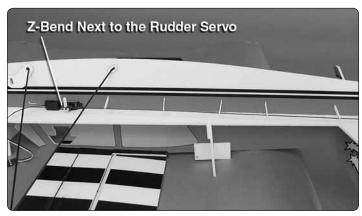
☐ 6. Insert the **rudder pushrod** from the front, through the five pushrod guides. The z-bend should be next to the rudder servo arm.
