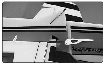
10. Slide the **black heat shrink tubing** over the aft end of the rudder pushrod. Insert the z-bend wire into the hole in the **rudder control horn** from the bottom. Slide the other end
