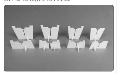
☐ 3. To prevent the parts from adhering to your building table, place a piece of waxed paper, or the clear plastic bag the parts came in, on your table. Use foam safe CA to glue the nine alignment crutch feet to the alignment crutches. Make sure the crutches and feet are flat against the building table and that the crutches are perpendicular to the table.
