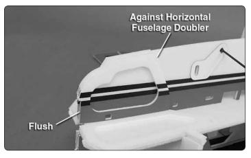
☐ 4. Glue the two **vertical fuselage doublers** to the front of the fuselage. Make sure they are flush with the front of the fuselage and against the horizontal fuselage doubler.
