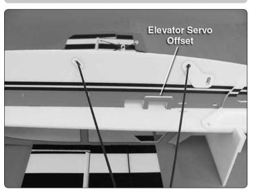
☐ 1. Use foam-safe CA to glue the **elevator servo offset** around the forward servo mounting hole on the left side of the fuselage.
