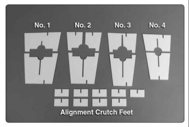
☐ 2. Remove the nine **fuselage alignment crutches** from the surrounding foam. **Note:** Use a sharp hobby knife to cut the crutch parts from the surrounding foam, trimming the tabs flush with the edges of the crutches.
