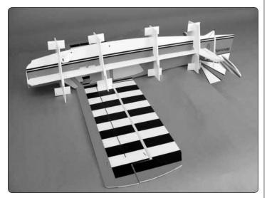
☐ 11. Place the **wing** upside down on the building table. Carefully turn the Citabria over and key the top of the fuselage into the bottom of the wing. Note that the vertical fin will need to hang over the edge of the building table. Check that #1, #3
