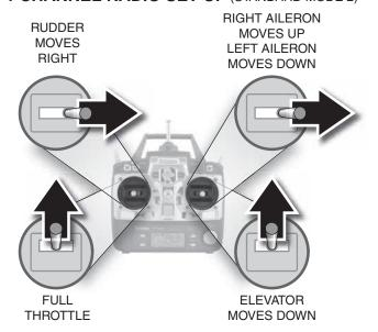
☐ 2. Make certain that the control surfaces respond in the correct direction as shown in the diagram. If any of the controls respond in the wrong direction, use the servo reversing in the transmitter to reverse the servos connected to those controls. Be certain the control surfaces have remained centered. Adjust if necessary.
