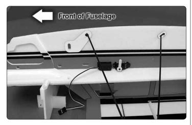
☐ 4. Center the servo arm on the rudder servo and trim off the extra servo arms. Use foam-safe CA to glue the rudder servo, with the output shaft forward, in the aft servo hole on the left side of the fuselage.
