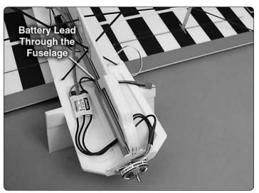
☐ 4. Place a piece of hook (rough) material under the fuselage, close to the front. Route the motor leads through the fuselage and connect them to the motor. Attach the ESC to the hook material.
