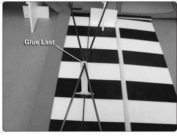
☐ 9. Once the glue has cured, glue the carbon rods to the brace supports.
