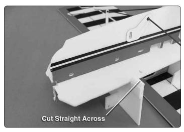
☐ 2. Turn the plane upside down. Use a sharp hobby knife to carefully cut the #1, #2 and #3 bottom crutches from the top crutches.
