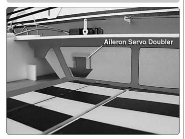
1. Use foam-safe CA to glue the **aileron servo doubler** to each side of the fuselage.
