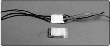
☐ 3. Place a small piece of loop (soft) side of the self adhesive hook and loop material to the back of the ESC and the receiver.
