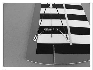
☐ 6. Check that all the carbon rods and brace doublers are in position and straight and the crutches are in position and flat on the building table. Start by gluing the carbon rod and the long brace doubler to the wing at the wing tip.
