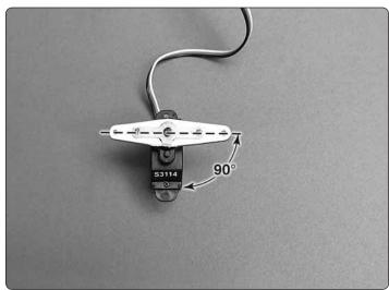
4. Install the aileron servo arm on the aileron servo. Make sure the servo arm is centered. Once the servo is installed, removal of the servo arm is difficult.
