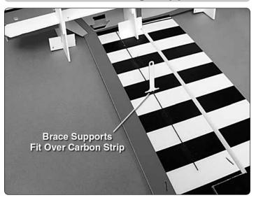
☐ 1. Locate the two **ABS** brace supports. There is a slot located in the center of each wing. Glue the ABS brace supports into the slots, perpendicular to the underside of the wing. It is possible that, during manufacturing, some glue may have gotten into the slot. If this has happened, **DO NOT FORCE** the supports into the slot. Use a sharp hobby knife to remove any excess glue.
