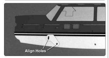
1. Locate the two **ABS landing gear supports**. Glue a landing gear support to each side of the fuselage in the location shown.
