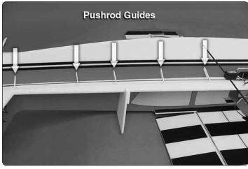
☐ 5. Install the pre-assembled elevator pushrod by inserting the ABS pushrod guides through the fuselage as shown. DO NOT glue the pushrod guides in place at this time.
