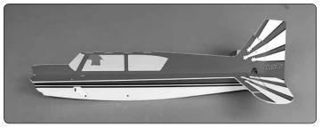
4. Insert the aft end of the horizontal fuselage into the front of the vertical fuselage. Key the horizontal and vertical fuselages together.
