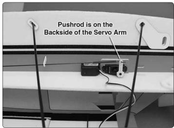
☐ 7. Remove the elevator servo arm and insert the z-bend into the outer hole of the arm, approximately 5/8" [16mm] from the center of the servo arm. **Note:** If you are not using a computer radio, and do not wish to set your model up with 3D control throws, you will need to insert the z-bend in a hole closer to the center of the servo arm. The z-bend should be installed so that the pushrod is on the back side of the servo
