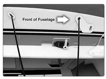
☐ 3. Install the elevator servo in the forward servo hole with the output shaft towards the front of the fuselage. Glue the servo in place with foam-safe CA. Be careful not to get any glue inside the servo case.
