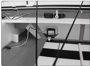
☐ 5. Use foam-safe CA to glue the aileron servo to the fuselage. Make sure the aileron servo wire is on the right side of the fuselage.
