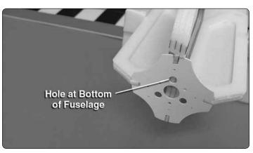
☐ 5. Glue the **ABS motor mount** to the front of the fuselage. Apply a bead of glue to the joint on all sides of the fuselage and motor mount. Take note of the orientation of the three large holes.
