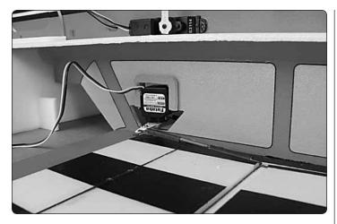
☐ 6. Insert the z-bend of both **aileron pushrods** in the aileron servo extension.
