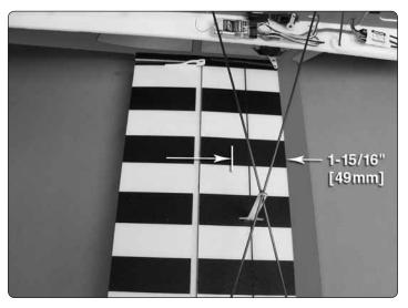
□ 1. Use a fine-point felt tip pen to mark lines on the bottom of the wing, 1-15/16" [49mm] from the leading edge of the wing, on both sides of the fuselage. Apply narrow (1/16" [1.5mm] strips of tape over the lines so you will be able to feel them when lifting the model with your fingers.
