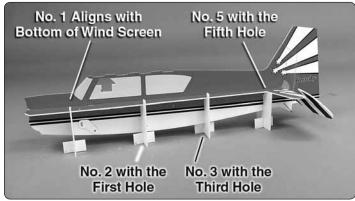
□ 5. On your building table, place the four bottom crutches with the feet on them underneath the fuselage in the locations shown. Crutch #1 is positioned in line with the bottom of the windscreen. Crutch #2 is positioned at the first hole in the side of the fuselage. Crutch #3 is positioned at the third hole in the side of the fuselage. Crutch #4 is positioned at the fifth hole in the side of the fuselage, just under the leading edge of the stabilizer.
