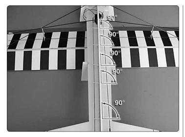
□ 6. Operate the rudder and elevator, checking that the pushrods do not bind in the pushrod guides. Adjust the position of the pushrod guides so that the pushrods are straight and the guides are 90 degrees to the fuselage. Glue the pushrod guides to the fuselage with foam-safe CA.
