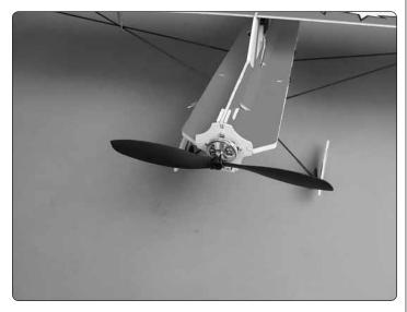
☐ 7. Install the propeller on the motor following the motor instructions.
