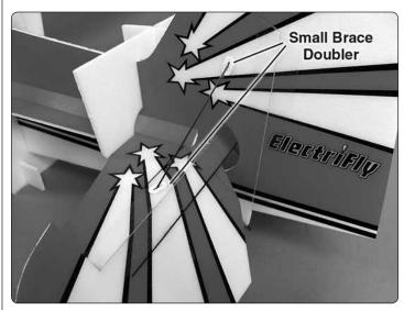
☐ 10. Turn the fuselage upright and position it on the crutches. Slide two **ABS small brace doublers** onto a 1 x 90mm carbon rod. Insert the carbon rod in the slot in the top of the stabilizer and the side of the vertical fin.
