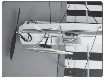
☐ 4. Apply the remaining hook and loop material to the bottom of the horizontal fuselage at the approximate location for the motor battery. Attach an opposite piece of hook and loop material to the battery. Trial fit the motor battery to the bottom of the fuselage and recheck the C.G.
