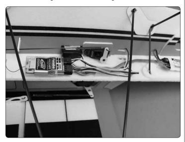
☐ 6. Position the receiver under the horizontal fuselage as far aft as possible. Make sure the servo wires do not interfere with the pushrods. Apply a piece of hook material on the bottom of the horizontal fuselage, at the receiver location. Attach the receiver to the fuselage. To prevent the wires from interfering with the pushrods, use a small piece of tape to attach them to the fuselage.
