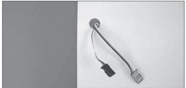
□ □ 13. Route the servo lead(s) through the hole in the top of the wing panel.
