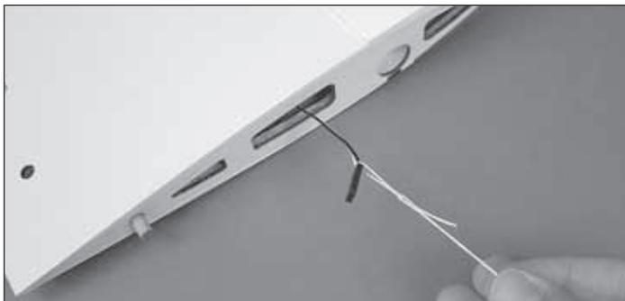
5. Use the string taped inside the **aileron servo bay** to pull the servo lead through the wing ribs.
