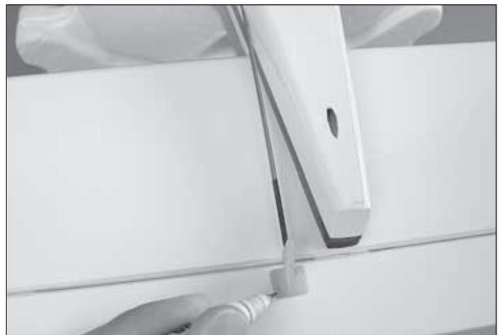
2. Temporarily insert a 36" [914mm] pushrod into the elevator outer pushrod tube that exits the right side of the fuselage. Use the position of the pushrod to mark the location for the elevator control horn onto the underside of the elevator.
