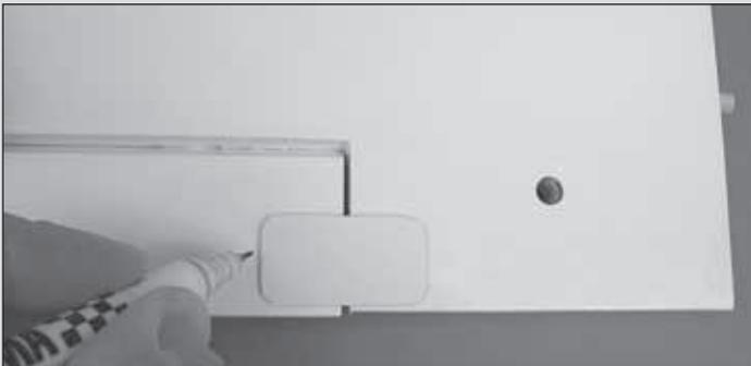
2. Center the strips over the inside edge of each flap just forward of the flap trailing edge. Use a felt-tip pen to trace around the shape of the ABS flap strips onto the flaps and wing panels.
