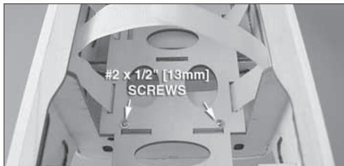
❑ 4. Fit the fuel tank tray into the fuselage by inserting the tab at the forward end of the tray into the slot in the firewall. Press the tray down onto the receiving tabs in the fuselage former and cross brace. Drill two 1/16" [1.6mm] holes through the tray and into the hardwood mounting blocks. Secure the tray in place using two #2 x 1/2" [13mm] screws and two #2 flat washers, being sure to harden the screw holes with thin CA.
