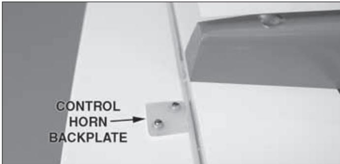
❑ 3. Drill 3/32" [2.4mm] holes at your marks completely through the elevator. Apply a couple drops of thin CA to each hole to harden the surrounding wood. Install a control horn and backplate onto the underside of the elevator using two 2-56 x 1/2" [13mm] machine screws.
