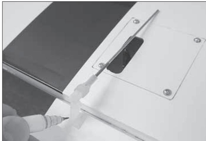
8. Position the control horn over the plywood plate in the aileron (if you cannot see it, hold the aileron at a shallow angle in good lighting or use a small pin to puncture the covering), using the position of the servo arm as a guide. Align the holes in the control horns directly over the aileron hinge line and mark the location of the control horn mounting holes.
