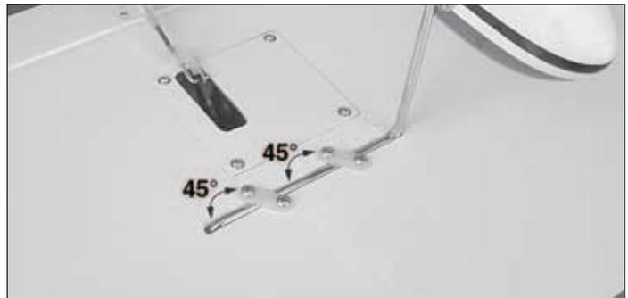
4. Fit the main landing gear legs into the slots in the underside of the wing panels. Position two nylon landing gear straps over each landing gear leg at a 45° angle as shown. Mark the locations of the screw holes onto the wing and drill holes at your marks using a 3/32" [2.4mm] drill bit. Secure the landing gear legs to the wing panels using the nylon landing gear straps and #4 x 1/2" [13mm] self-tapping screws.
