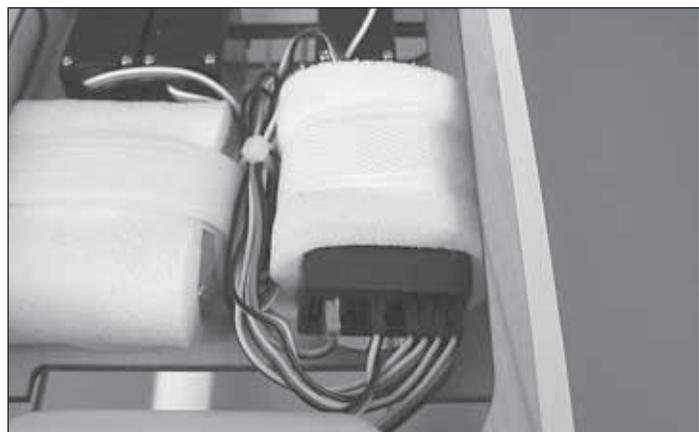
❑ 2. Connect the servos to the receiver, being sure that the leads will not interfere with the tail pushrods. Depending on the ESC being used (if applicable), you may need a servo extension to reach the receiver. If you plan to connect the flap and aileron servos to the receiver using Y-harnesses, connect the harnesses to the receiver at this time.
