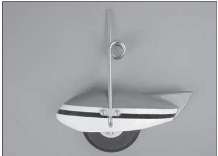
5. Install the nose wheel pant and wheel onto the nose gear wire in the same manner as you did the main landing gear.
