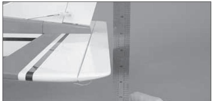
Use a Great Planes AccuThrow™ (or a ruler) to accurately measure and set the control throw of each control surface as indicated in the chart that follows. If your radio does not have dual rates, we recommend setting the throws at the low rate setting.
