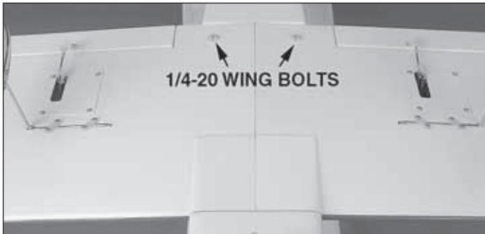
1. Fit the two wing panels onto the aluminum **wing joiner tube**. Slide the root ribs of the panels together so that the **anti-rotation pin** preinstalled in one panel fits into the mating hole of the other panel. Slide the wing dowels that are preinstalled in the LE of the wing panels into the receiving holes in the fuselage at the front of the **wing saddle**. Use two 1/4-20 nylon wing bolts to secure the wing in place.
