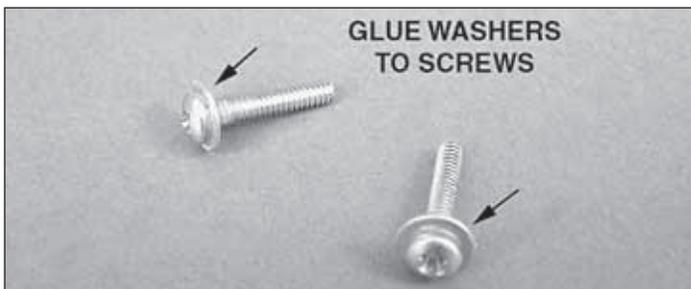
2. We suggest gluing a #4 washer to each of the two 4-40 x 5/8" [16mm] canopy hatch screws. Take care not to get glue onto the threads of the screws. This will make the screws easier to work with at the flying field.
