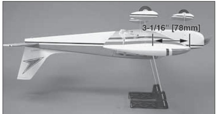
☐ 2. With the wing attached to the fuselage, all parts of the model installed (ready to fly) and an empty fuel tank, place the model upside-down on a Great Planes C.G. Machine, or lift it upside-down at the balance point you marked.
