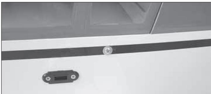
3. Fit the **canopy hatch** in place by inserting the two dowel pins into the receiving holes at the front of the hatch opening. Use the two 4-40 x 5/8" [16mm] machine screws to secure the hatch in place.
