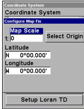
**Configure a map fix so the unit can find your position on a printed chart or topographical map.**
