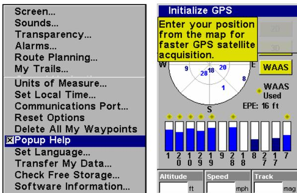
System Setup Menu (left) with Pop-up Help command highlighted. The second example (right) shows the Pop-up Help message for the Initialize GPS command, located on the Status Page menu.
