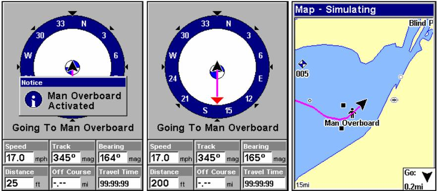
Navigating to Man Overboard: "Man Overboard activated" message (left). The Navigation Page (center) with Map Page (right). The victim is astern of the vessel; the GPS shows which direction to steer to for the rescue.
