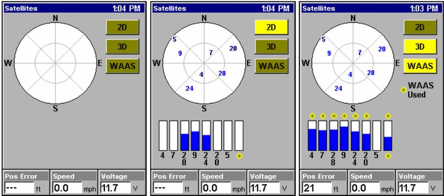
**Satellite Status Page.** The first image (left) indicates unit has not locked on to any satellites and has no fix on its position. The second image (center) shows satellites being scanned. The third image (right) shows satellite lock-on with 3D position acquired (latitude, longitude and altitude), and WAAS reception.
