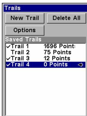
New trail, named "Trail 4," is created when Trail 3 is made inactive. Any new travel will be recorded in this trail, which is active and visible. Trails do not need to be visible in order to be active.
