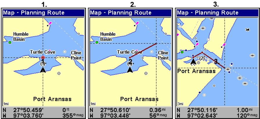
Route creation sequence (left to right): Fig. 1. Set route waypoint (1) at the cove entrance. Fig. 2. Move cursor northeast to set point (2) at channel entrance. Fig. 3. With point (2) set, move cursor southeast to mark channel exit with waypoint (3). In figures 2 and 3, notice the rubber band line extending from the previously set waypoint to the cursor. This line will become the course for the route.
