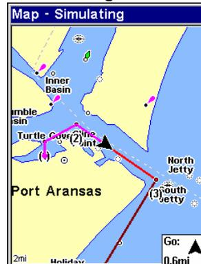
In Fig. 3 the traveler has turned northeast on his new course and is heading straight for Wpt 2, which is 0.27 miles away. Fig. 4 shows route navigation on the Map Page. In this figure, the traveler has reached Wpt 2 and is starting on the leg between Wpts 2 and 3.
