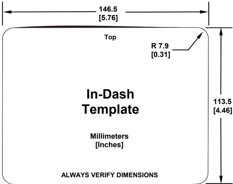
**In-dash mounting template for the GlobalMap 5150c, showing dimensions. NOTE: The figure above is *not* printed to scale. a scaled template (FM-5 In-Dash Adapter Kit instructions) is available for free download from our web site, [www.lowrance.com](http://www.lowrance.com).**
