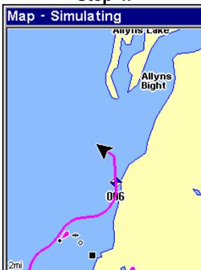
Sequence for setting a waypoint. Step 1: while traveling, *quickly* press **WPT** twice to call up Find Waypoint screen (seen in Step 2) and set a point. Step 3: message says the waypoint has been saved. Step 4: vehicle continues on its way; number waypoint symbol is visible on map.
