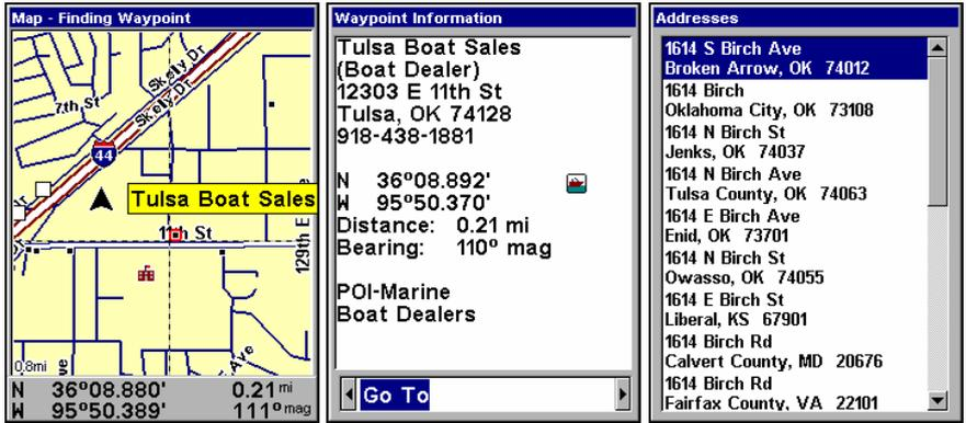
Map Page showing location of the address on the map, highlighted by cursor (left). This address is a business in the POI database, so you can display the POI information window, then navigate to it (center). This address is not in the POI database (right), so the Waypoint key will not display any information for this address.
