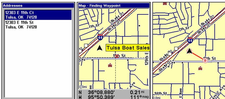
**Address search result list (left). Map Page showing location of the address on the map (center) highlighted by cursor. After the address is located, you can navigate to it ("D" symbol for destination) (right).**
