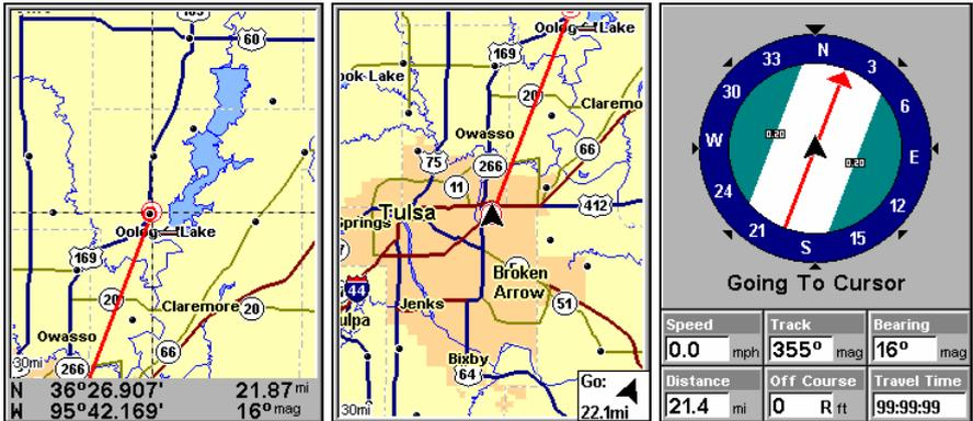
The first figure (left) clearly shows the red course line connecting your current position to your destination. The 30-mile zoom (center), shows both current position and direction to destination on screen. The Navigation Page (right) will also show navigation information.
