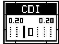
The CDI's range shows beneath the CDI label. On the above screen, the CDI range is .20 mile, which is the default. You can adjust the range by selecting the "ALARMS/CDI" label on the main menu. This is also shown by the dotted lines at the far left and right side of the CDI. If the solid line is on either of the dotted lines, then you are 0.20 mile off course. Remember, if the line moves to the left, then you are too far to the right of the desired course line and vice-versa.
