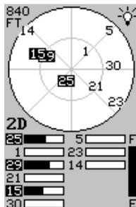
The GPS receiver is tracking satellites that are surrounded by a black box. If the satellite number is not surrounded by a box, then the receiver hasn't locked onto that satellite and it isn't being used to solve the position.
