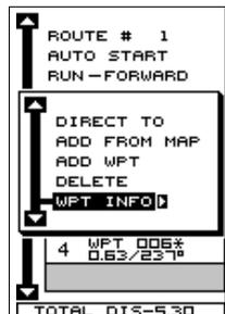
The selected waypoint number appears at the top of this screen. Information about the waypoint shows at the bottom of the screen. When you're finished with this screen, press the EXIT key to erase it.
