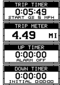
The up timer starts at zero and counts up. The up timer also has an alarm. The down timer starts from a user setting and counts down to zero.
