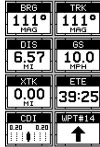
This screen is composed of eight digital boxes. Track (TRK) and ground speed (GS) data are all that show if you're not navigating to a waypoint. If you are navigating to a waypoint, then bearing (BRG), distance to waypoint (DIS), estimated time en route (ETE), cross track error (XTK), destination arrow, and the CDI also show.
