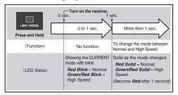
Please check the operation mode by observing the LED when turning on the receiver. The best way to confirm the mode you are on is to make sure that there are no other FASST transmitters turned on around you.
