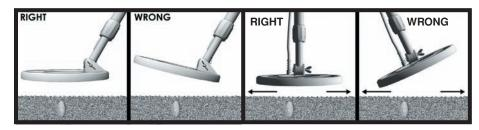
Keep the search coil as close to the ground as possible for greater penetration, and make sure the search coil remains parallel to the ground as you search.
