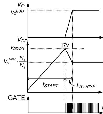
**Figure 14. Typical Startup Waveform**
