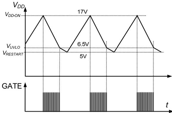
**Figure 15.  $V_{DD}$  UVLO at Normal Mode**
