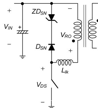
**Figure 11. TVS Snubber Circuitry**
