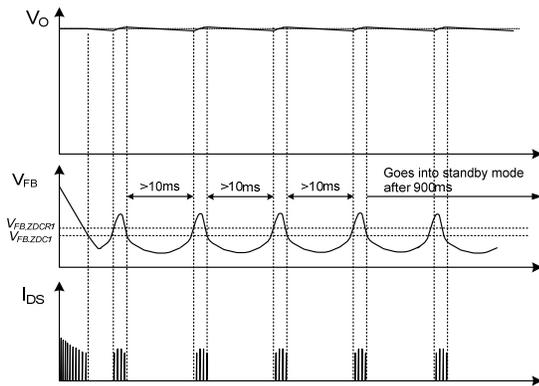
**Figure 9. Timing Diagram for Entering Standby Mode**
