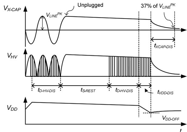
**Figure 17. Timing Diagram for AX-CAP™ Discharge**
