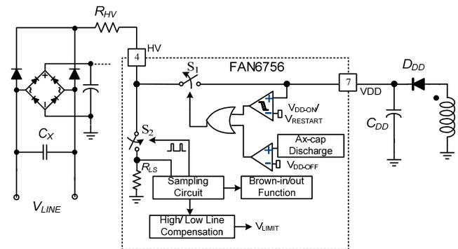
**Figure 5. HV Pin Functional Block Diagram****Define Parameter:**
