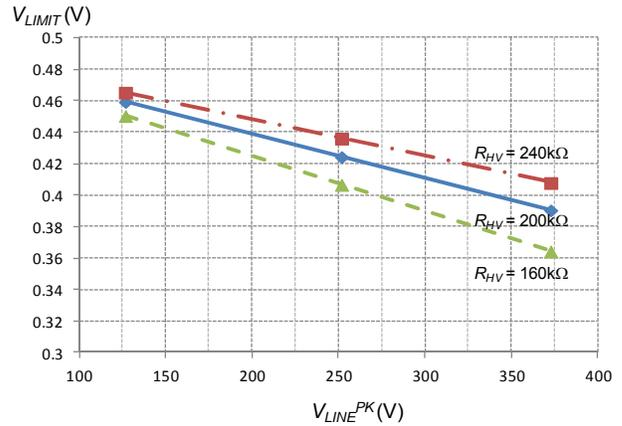
**Figure 13. Current Limit vs. Line Voltage**
