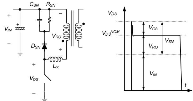
**Figure 10. Typical RCD Snubber Circuit and  $V_{DS}$  Waveform**
