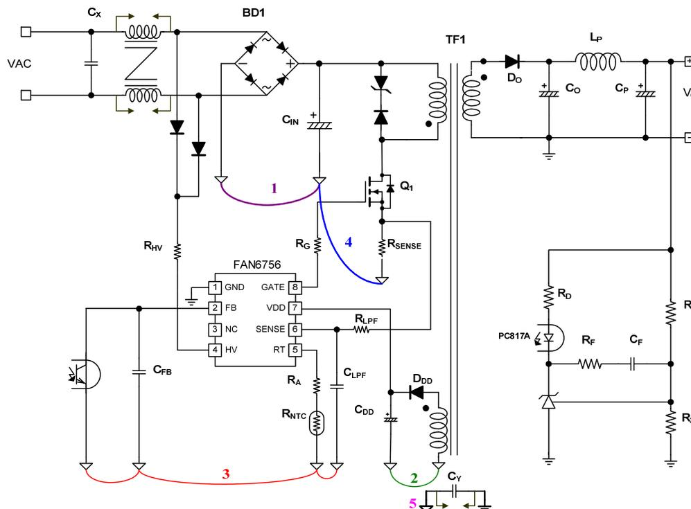
Figure 23. Grounding PCB Layout Diagram
