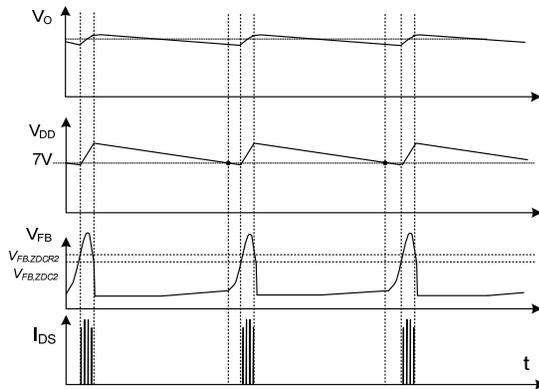
**Figure 16. Deep Burst Operation in Standby Mode****Design Example:**
