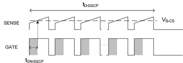
Figure 20. SSCP Detection Waveform
