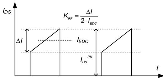
**Figure 4. Typical MOSFET Current Waveform****Design Tips:**
