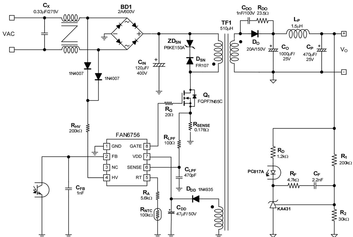
**Figure 22. Final Schematic of Design Example**
