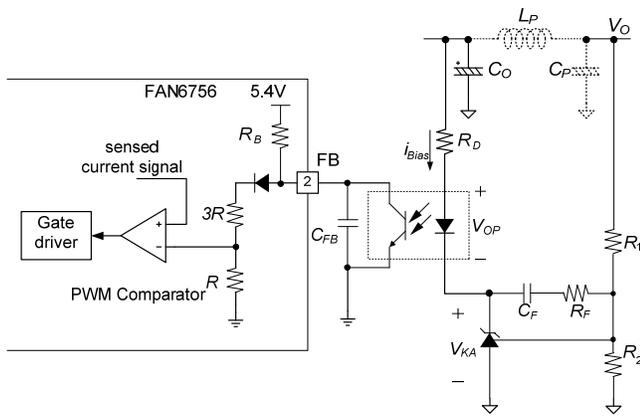
**Figure 8. Feedback Compensation Network**
