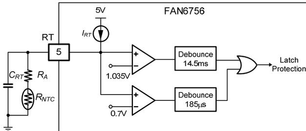
Figure 18. Thermal Protection Circuit
