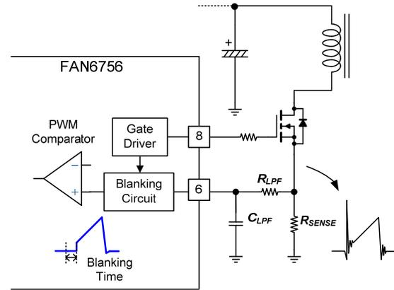
Figure 19. Current-Sensing Circuit and Waveform
