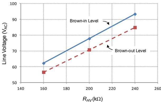
**Figure 12. Brown-in/out Level with Different  $R_{HV}$**
