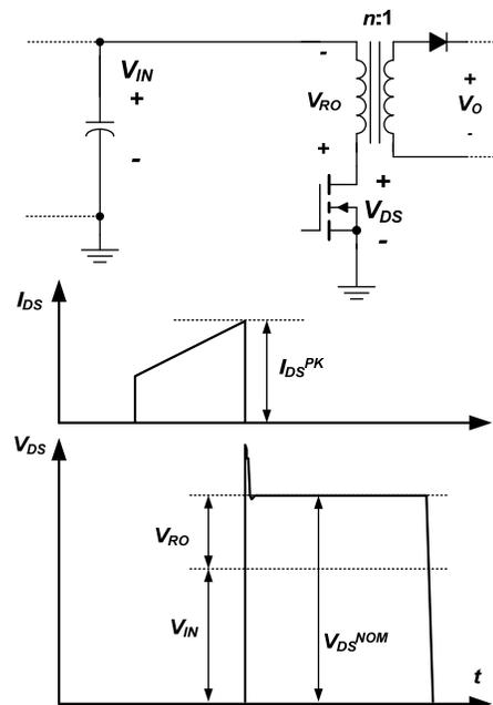
Figure 3. Typical MOSFET  $V_{DS}$  Waveform
