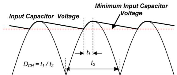
Figure 2. Input Capacitor Voltage Waveform
