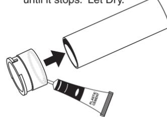
**C.** Apply plastic cement inside front of Engine Mount Tube. Insert Upper Ring. Let Dry.
