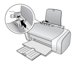
3. Insert the paper, printable side up, against the right edge guide. Then slide the left edge guide against the paper (but not too tightly).
