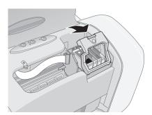
6. Squeeze the back tab of the used cartridge and lift it out of the printer. Don't take the cartridge apart or try to refill it.
