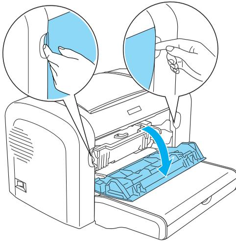
3. Remove the developer cartridge.
