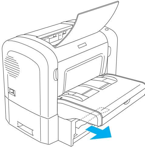
3. Remove all paper from the paper tray and press down on the plate until it locks into position.
