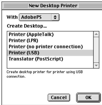
3. Click Change under USB Printer Selection in the dialog box that appears to select the printer. The dialog box shown below will be displayed, showing a list of connected USB printers. Select the EPL-6200 printer from the list, and then click OK.
