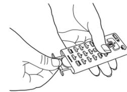
Remember to pull out the clear plastic tab from the battery compartment before using the remote.
