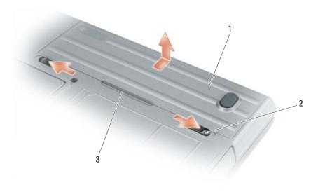
battery battery-bay latch releases (2) 3 battery tab
