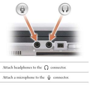
**IEEE 1394 CONNECTOR** — Connects devices supporting IEEE 1394 high-speed transfer rates, such as some digital video cameras.
