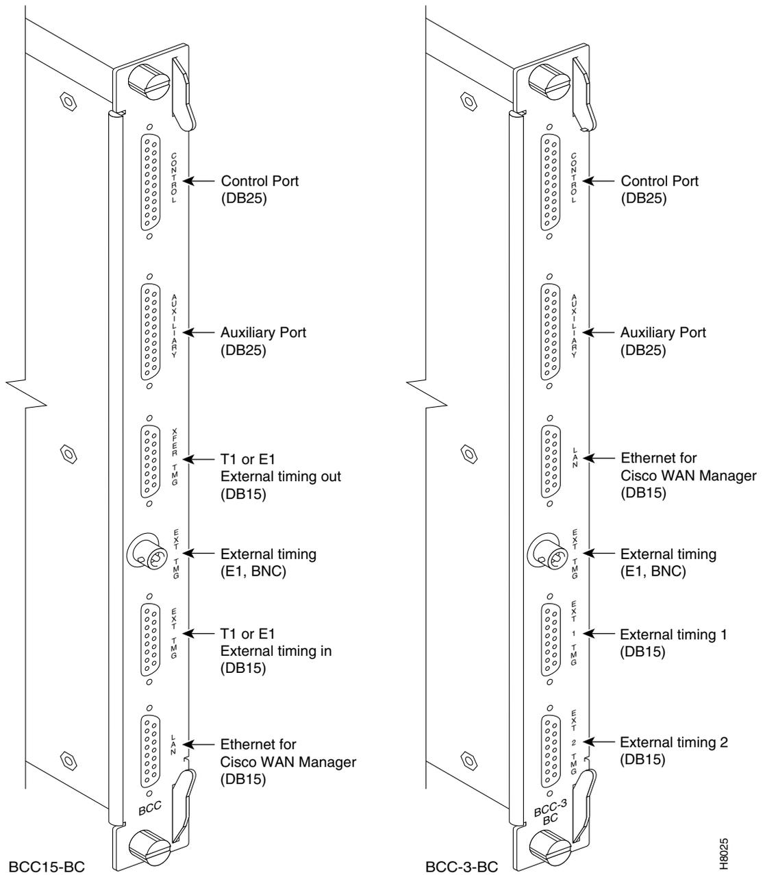
Another function of the line module back card is to provide two low-speed, serial communications ports (Table 3-3). The first port (CONTROL) is a bidirectional port used for connecting the BPX to a local terminal or to a modem for a remote terminal “dial-in” connection. The second port (AUXILIARY) is an output only and is typically used to connect to a log printer.
