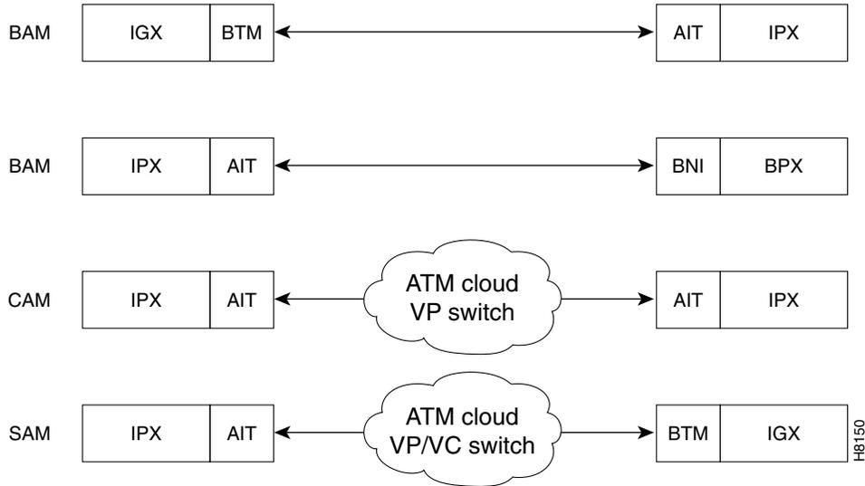
Note: IPX with AIT card are interchangeable with IGX with BTM card in this diagram.
