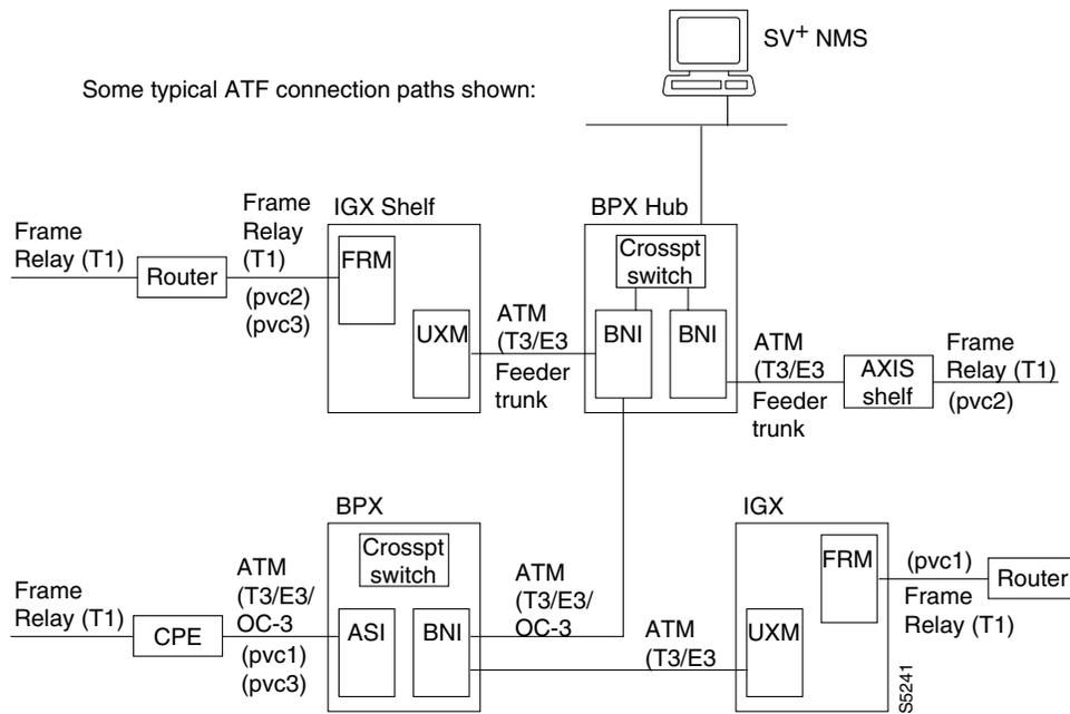
The cells within the frame are expected to possess the standard ATM Access Interface cell header. The traffic is assumed to have AAL-5 PDUs, and will not function properly otherwise (framing errors will result). Within the AAL-5 PDUs, the data must be packaged in standard Frame Relay frames, one frame per PDU (with respect to the AAL-5 layer).
