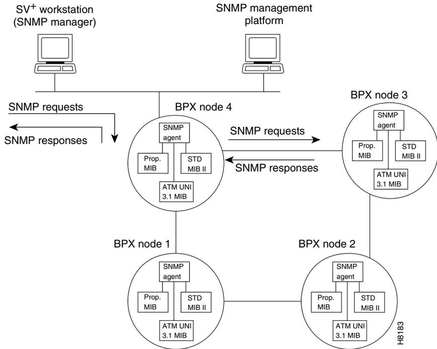
Communication between the agents and the SNMP manager uses the standard UDP protocol encapsulated within IP protocol. The communication link between the SNMP manager and the directly attached BPX node uses the Ethernet interface of an BCC processor card. The SNMP manager can be either local or remote to the BPX node.
