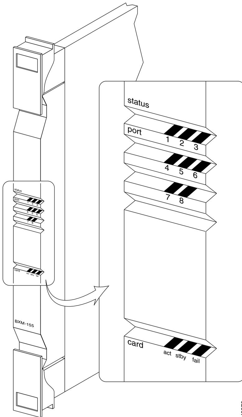
Figure 6-4 BXM-T3/E3 Front Panel, 12-Port Card Shown
