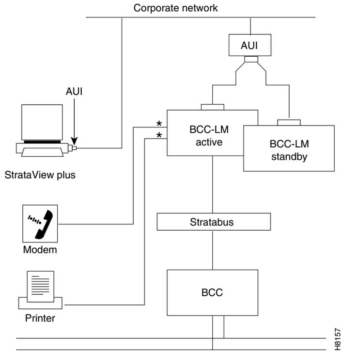
Two ports on BCC-LM can be used to connect up to two (2) of the peripherals shown.
