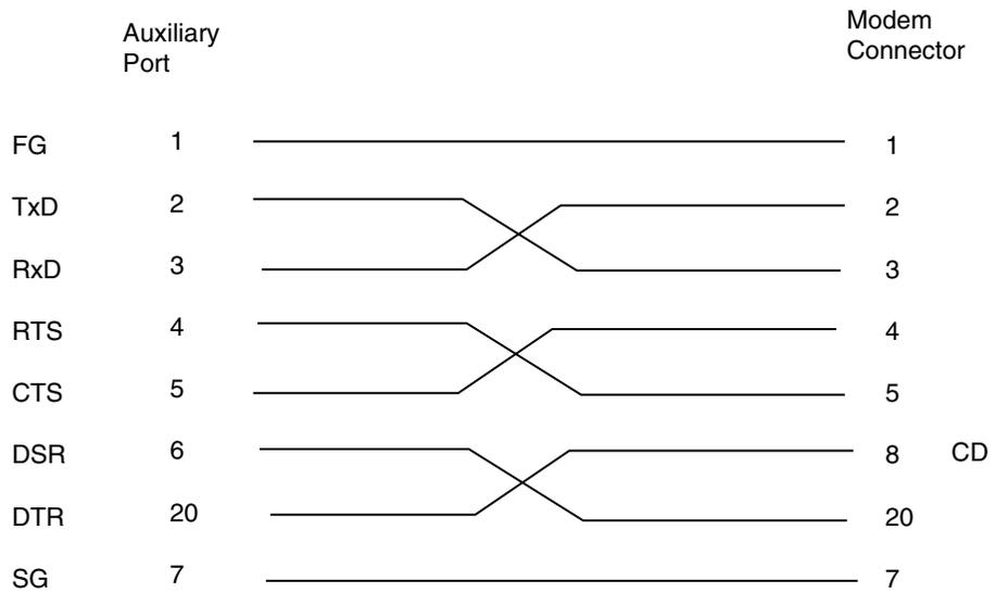
Note: Cable must be connected in direction shown from node to modem because wiring is not pin-to-pin symmetrical.
