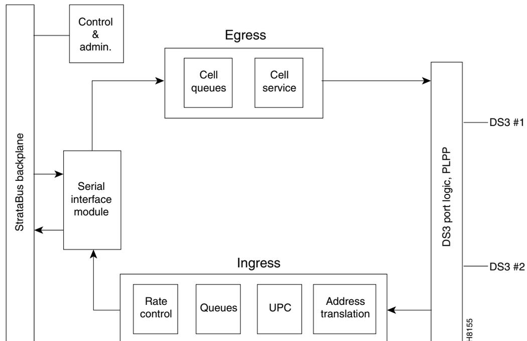
Each port provides an aggregate ATM connection bandwidth of 96,000 cells/second (T3) or 80,000 cells/sec (E3), or 353,208 cells/sec (OC3).
