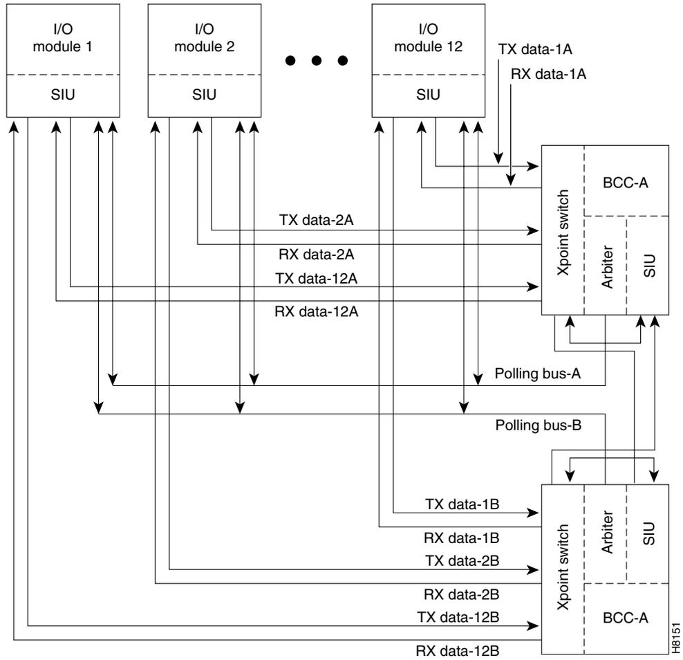
Figure 3-3 BCC-4 Block Diagram
