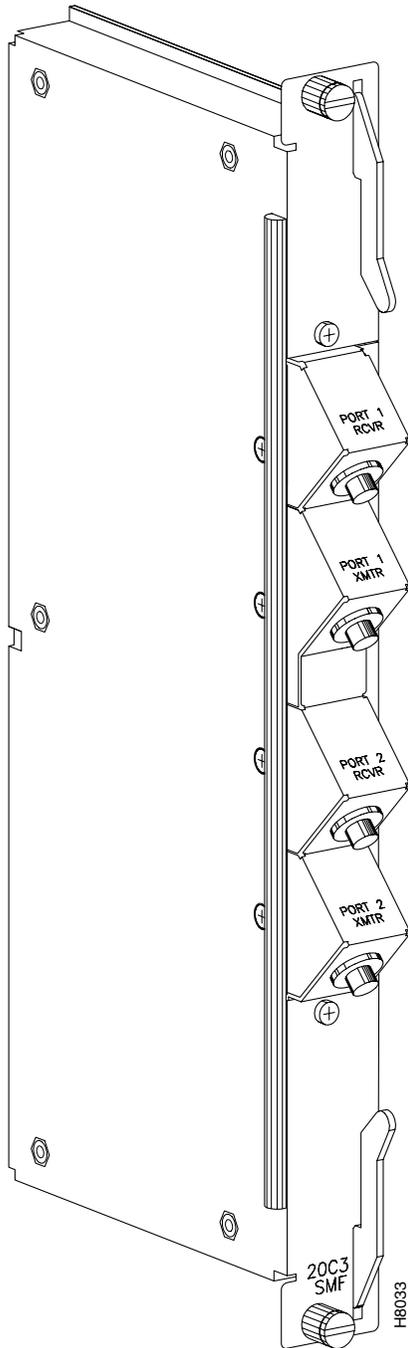
Figure 4-9 LM-OC3-MMF Face Plate
