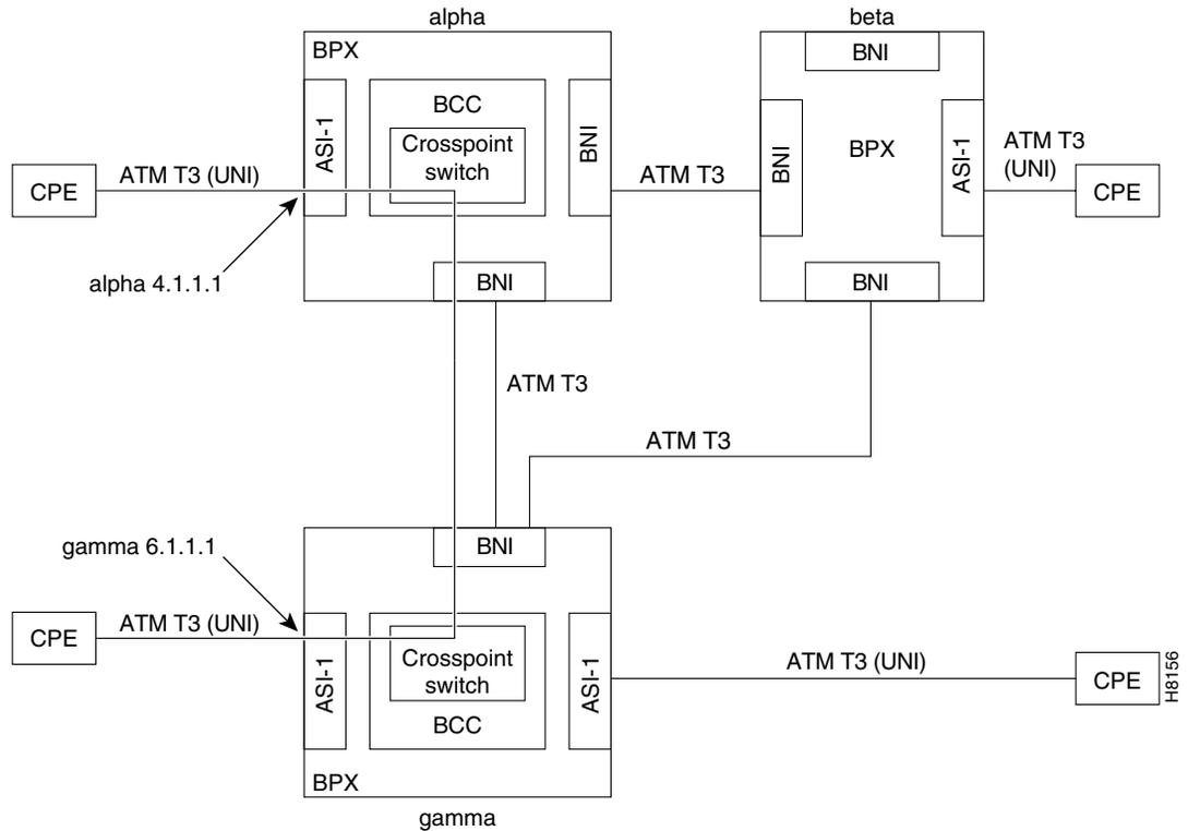
at alpha: addcon 4.1.1.1 gamma 6.1.1.1 [connection parameters...]
