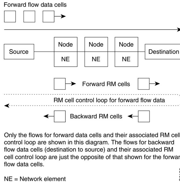
Only the flows for forward data cells and their associated RM cell control loop are shown in this diagram. The flows for backward flow data cells (destination to source) and their associated RM cell control loop are just the opposite of that shown for the forward flow data cells.
