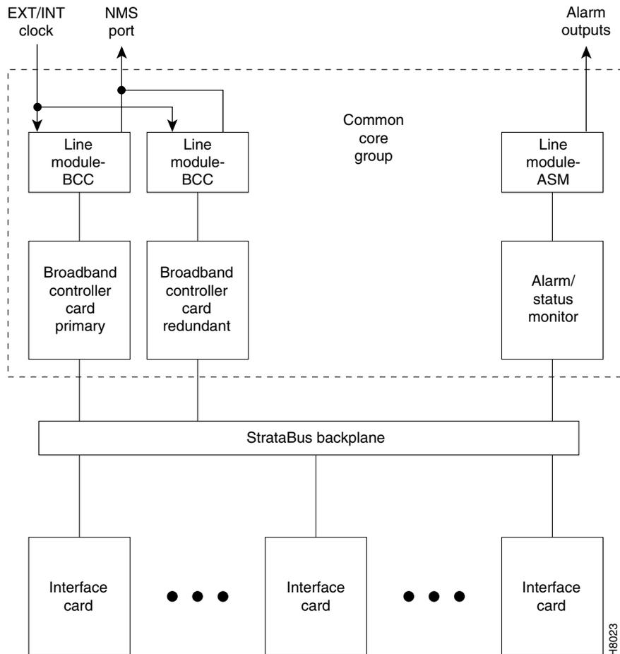
The BCC-3 and BCC-32 are functionally equivalent and the BCC-4 is similar except for some additional features such as support of 19.6 Gbps operation. The term BCC is used in this manual to refer to the functional operation of the Broadband Controller Card. When a difference in operation does occur, the specific type of BCC is specified. This card group (see Figure 3-1) provides the following functions:
