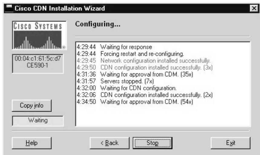
After you click **Finish** in the Installation Wizard, a status box appears with configuration information. Ultimately, you see the device status as “online.” However, if the device is a new Content Engine or Content Router, or if it previously existed but was moved to a different Content Distribution Manager administrative domain, then it must first be approved within the Content Distribution Manager GUI before the device status changes to online.
