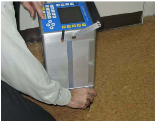
Figure 3-6 - Leveling the Tripod using the Right Hand Footscrew
