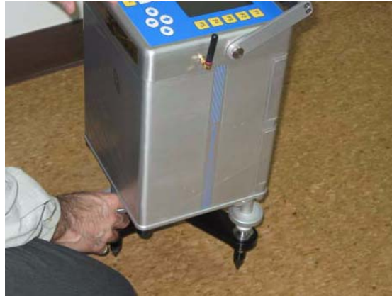
Figure 3-7 - Leveling the Tripod using the Front Footscrew
