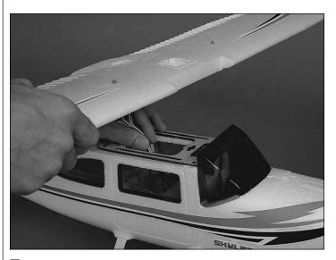
☐ 4. Dropping the wing into position, guide the servo wires coming from the bottom of the wing down past the elevator and rudder servos and out the bottom of the fuselage. Be certain none of the wires get caught between the bottom of the wing and the fuselage.
