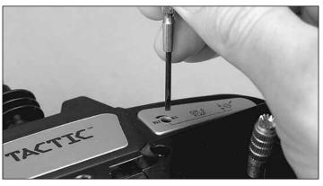
4. Measure and set the rest of the throws the same way. When setting the flap throw, if using the Tactic radio suggested, use the adjustment screw in the front of the transmitter to change the throw.
