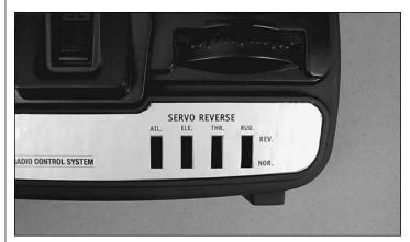
□ 9. Move the elevator stick on the transmitter up and down to make sure the elevator responds smoothly and in the correct direction. If the elevator responds the wrong way, switch the elevator servo reversing switch on the transmitter.
