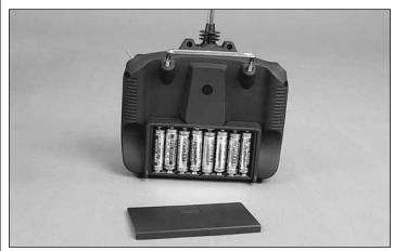
■ 3. Install the batteries in your transmitter.
