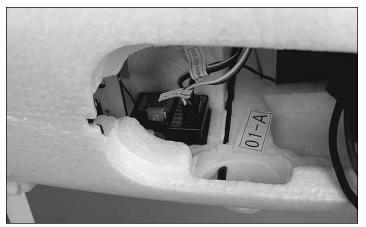
□ 2. Place a 1" [25.4mm] patch of double-sided adhesive foam tape (not included) on the bottom of the receiver. Temporarily place the receiver into its molded-in *cubby* in the fuselage (but don't remove the backing from the adhesive foam tape on the back of the receiver yet—there will be more wires to connect later when mounting the wing).
