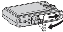
2. Load the battery into the camera.
