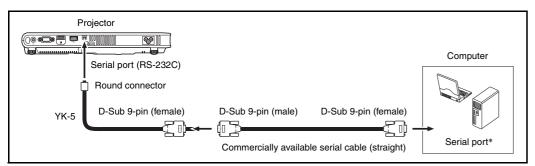
\* A D-Sub 9-pin (male) type connector is standard for computer serial ports, but there may be cases where the shape of a particular computer's connector is different. For details about connecting a commercially available serial cable to your computer, see the user documentation that comes with it.
