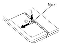
3 Press the memory card to unlock and the card will release. Pull the card out and remove.
