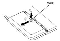
Insert and push a pin into the hole of the Reset key.
