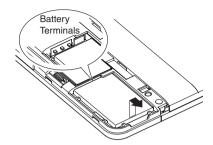
5 Securely insert a new battery into the unit ensuring the terminals make contact.
