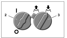
The rotational direction switch **3** must be turned to the right. The feed funnel **1** must be empty.
