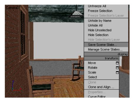
**3** In the Save Scene State dialog box, select all the scene parts so that cameras, environment, layers, lights, materials and object properties will be saved with the scene state.
