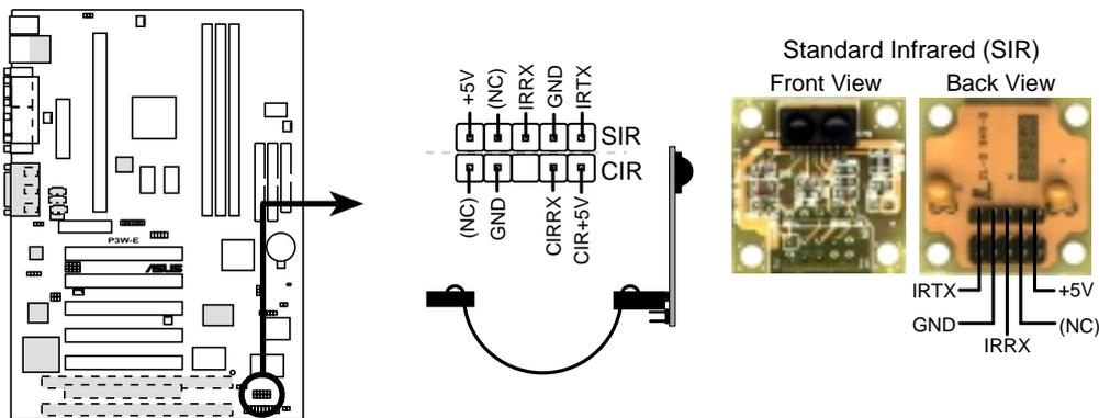
P3W-E Infrared Module Connector
