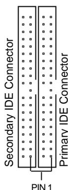
**NOTE:** Orient the red markings on the IDE ribbon cable to PIN 1
