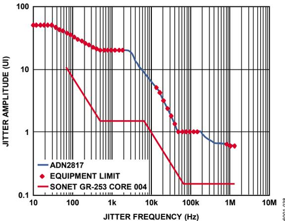
Figure 11. Jitter Tolerance, OC-3
