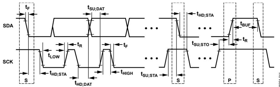
Figure 22. I<sup>2</sup>C Port Timing Diagram
