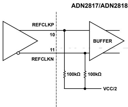
Figure 33. Differential REFCLK Configuration
