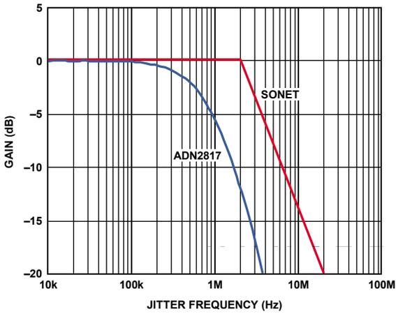
Figure 13. Jitter Transfer, OC-48
