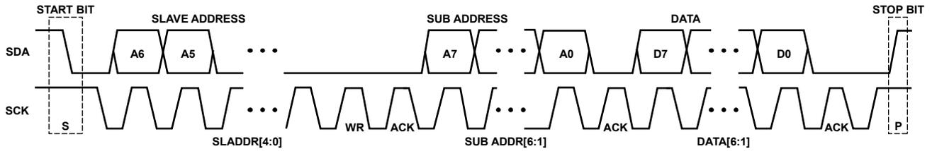
Figure 21. I<sup>2</sup>C Data Transfer Timing
