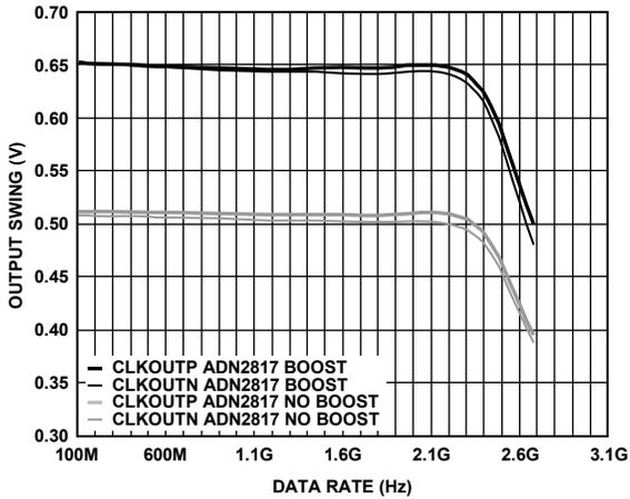
Figure 14. Output Swing vs. Data Rate
