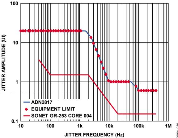
Figure 10. Jitter Tolerance, OC-1
