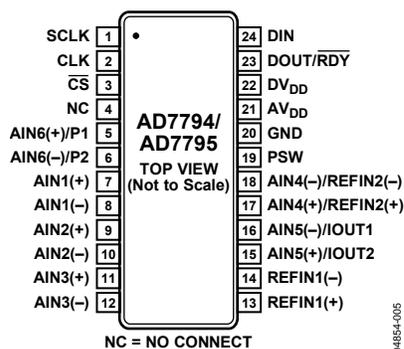
Figure 5. Pin Configuration
