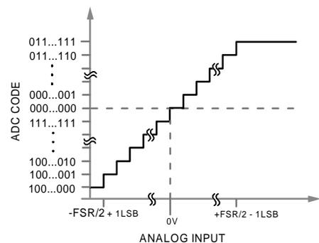
Figure 6. Transfer Characteristic
