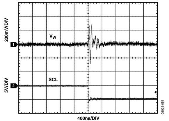
Figure 29. Digital Feedthrough
