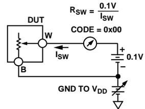
Figure 37. Test Circuit for Common-Mode Leakage Current
