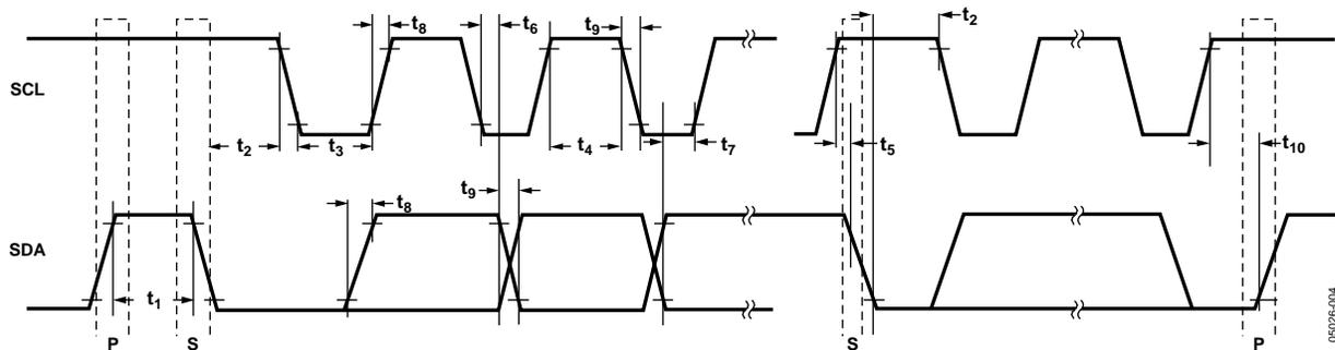
Figure 4. I<sup>2</sup>C Interface Timing Diagram
