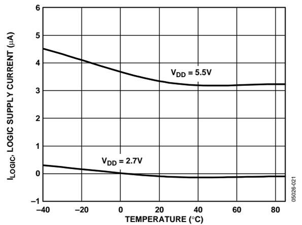
Figure 17. Logic Supply Current vs. Temperature vs. V<sub>DD</sub>
