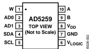
Figure 3. Pinout
