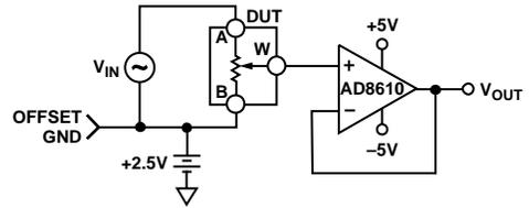
Figure 36. Test Circuit for Gain vs. Frequency
