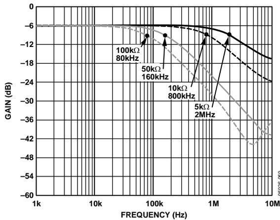
Figure 26. -3 dB Bandwidth @ Code = 0x80
