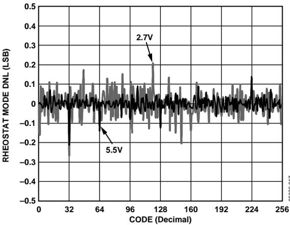
Figure 7. R-DNL vs. Code vs. Supply Voltage
