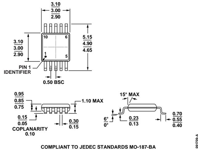
Figure 48. 10-Lead Mini Small Outline Package [MSOP] (RM-10)
