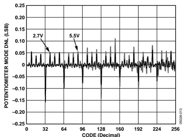
Figure 11. DNL vs. Code vs. Supply Voltage
