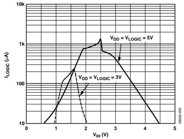
Figure 27. Logic Supply Current vs. Input Voltage
