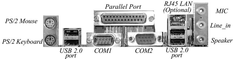
Figure 3: I/O back panel layout
