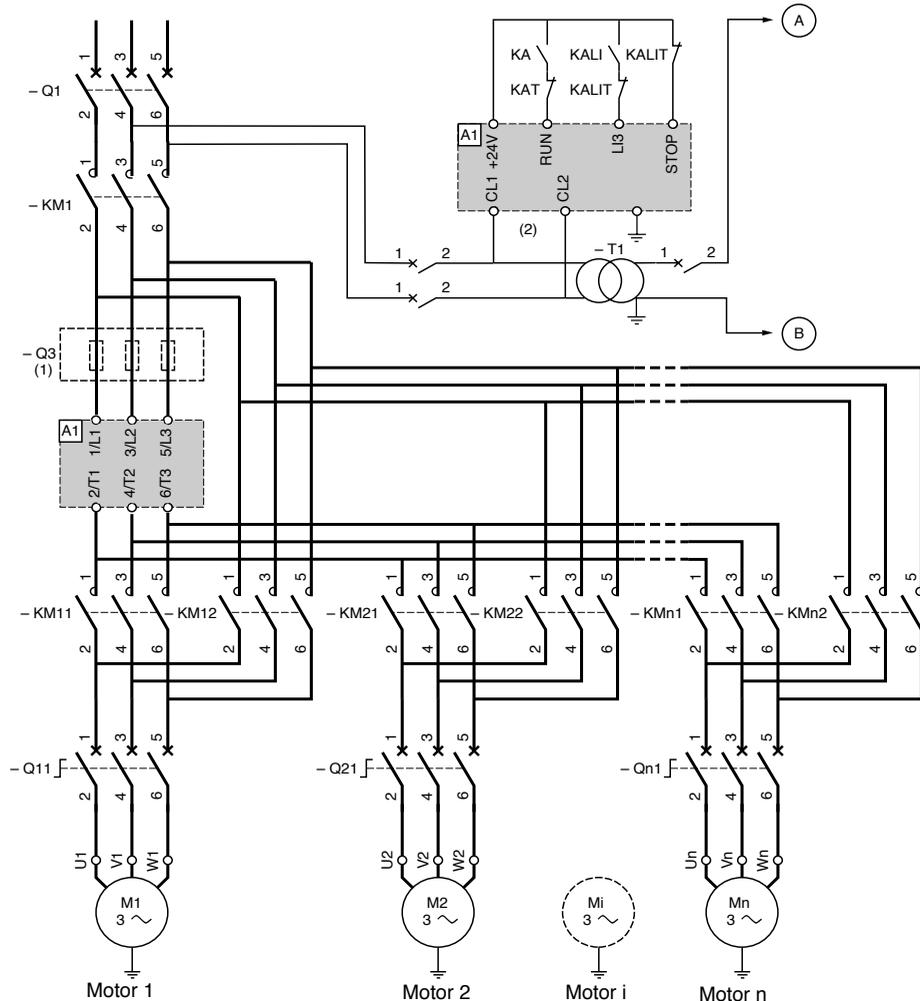
(1) Installation of fuses for type 2 coordination (conforming to IEC 60 947-4-2)
