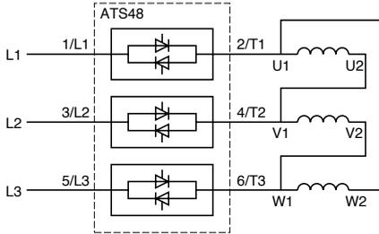
The motor connection depends on the supply voltage, **which in this example is a delta connection.**
