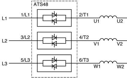
The motor connection depends on the supply voltage, **which in this example is a star connection.**
