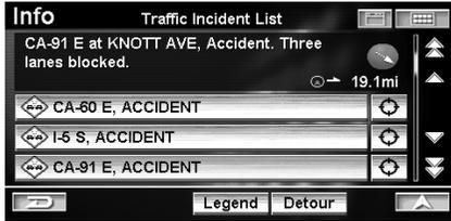
The system analyzes traffic data reported on the route within 30 miles of the vehicle’s position. If traffic congestion is found, the system displays a message with the distance to the congestion, and the anticipated delay if the congestion is not detoured.
