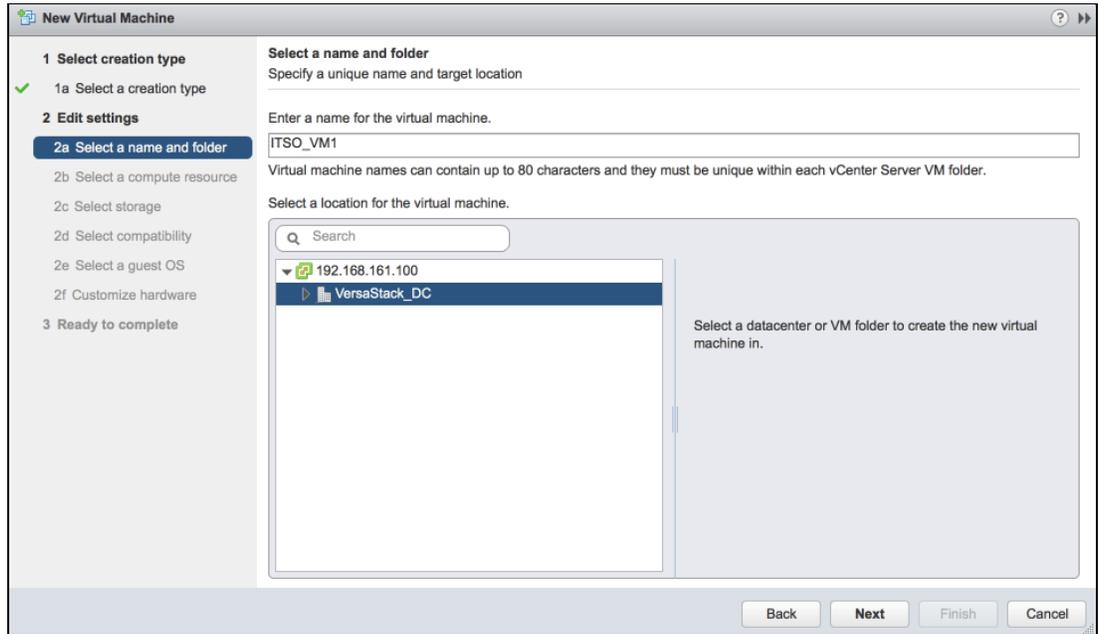
Figure 7-39 Select virtual machine name and folder
