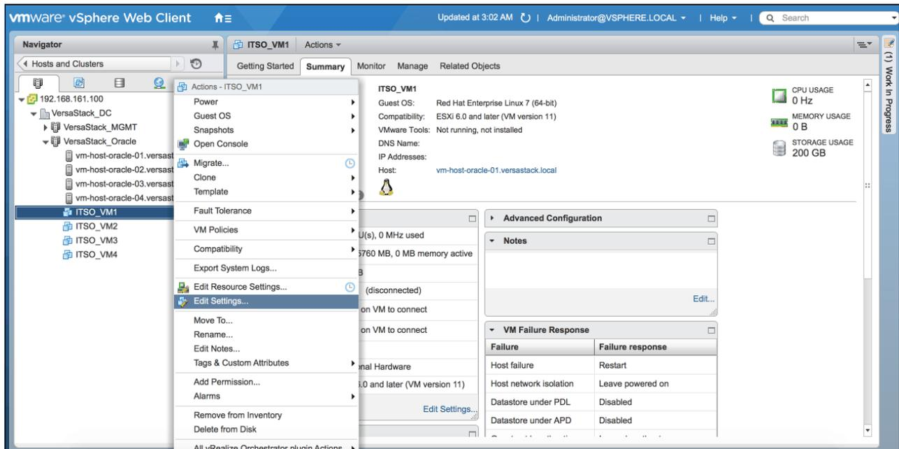
Figure 7-47 Edit virtual machine settings
