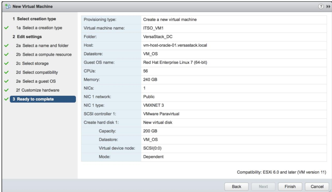
Figure 7-46 Review virtual machine configuration
