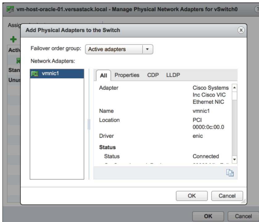
Figure 7-25 Add physical adapters to the Switch
