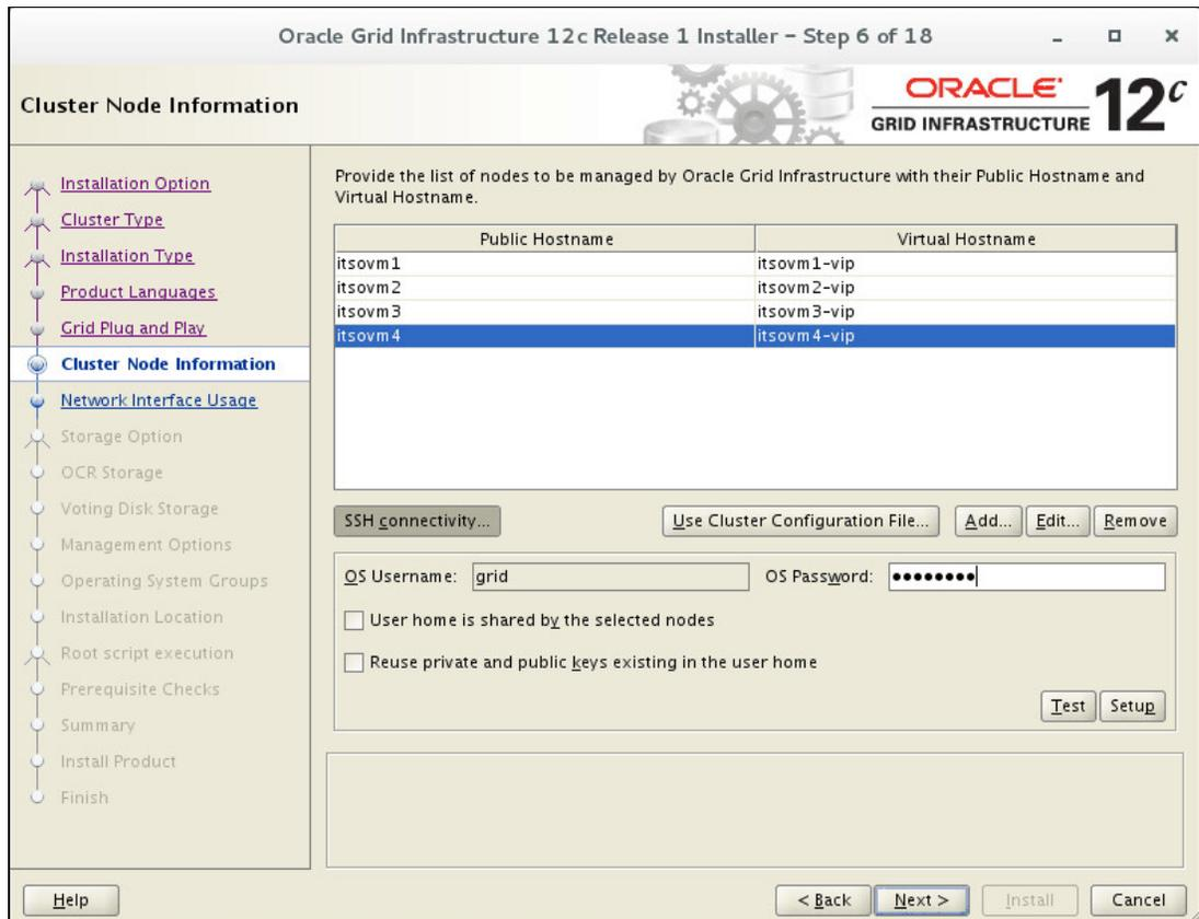
Figure 8-12 Setup passwordless SSH connectivity for grid user
