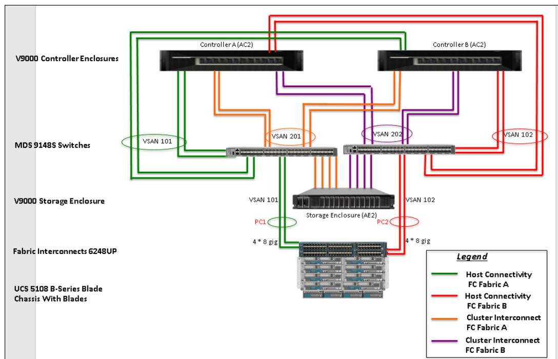
Figure 5-1 VersaStack cabling diagram
