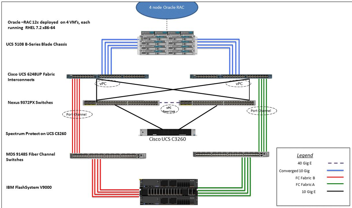
Figure 2-2 Oracle-RAC built on VersaStack
