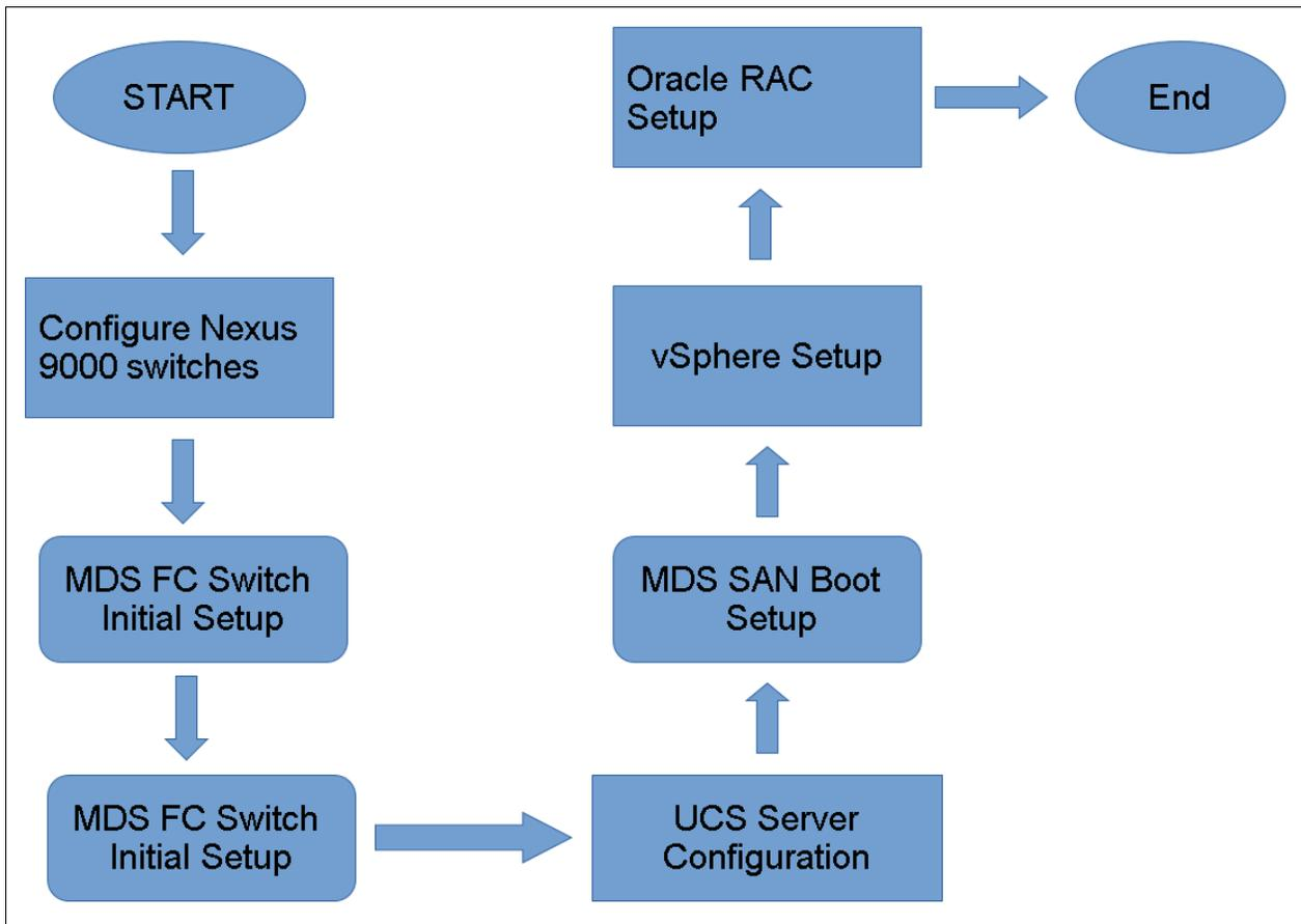
Figure 5-3 VersaStack build process
