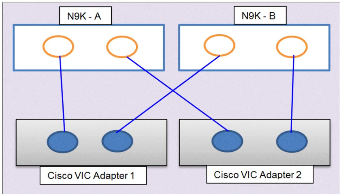
Figure 2-6 Nexus 9k switches to Cisco C3260 connectivity
