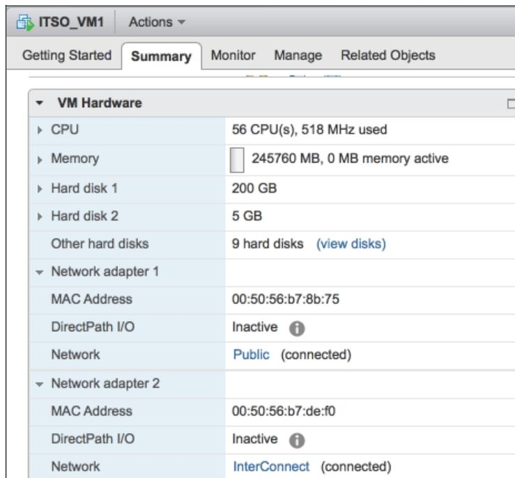
Figure 8-1 Check MAC Addresses of Ethernet interfaces
