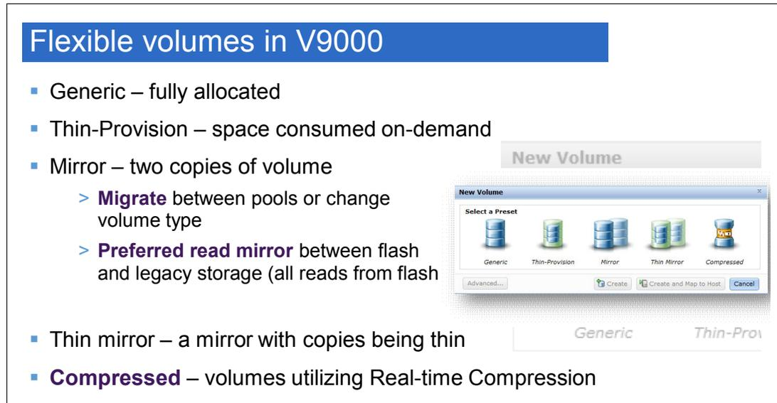
Figure 4-2 Flexible volumes in FlashSystem V9000
