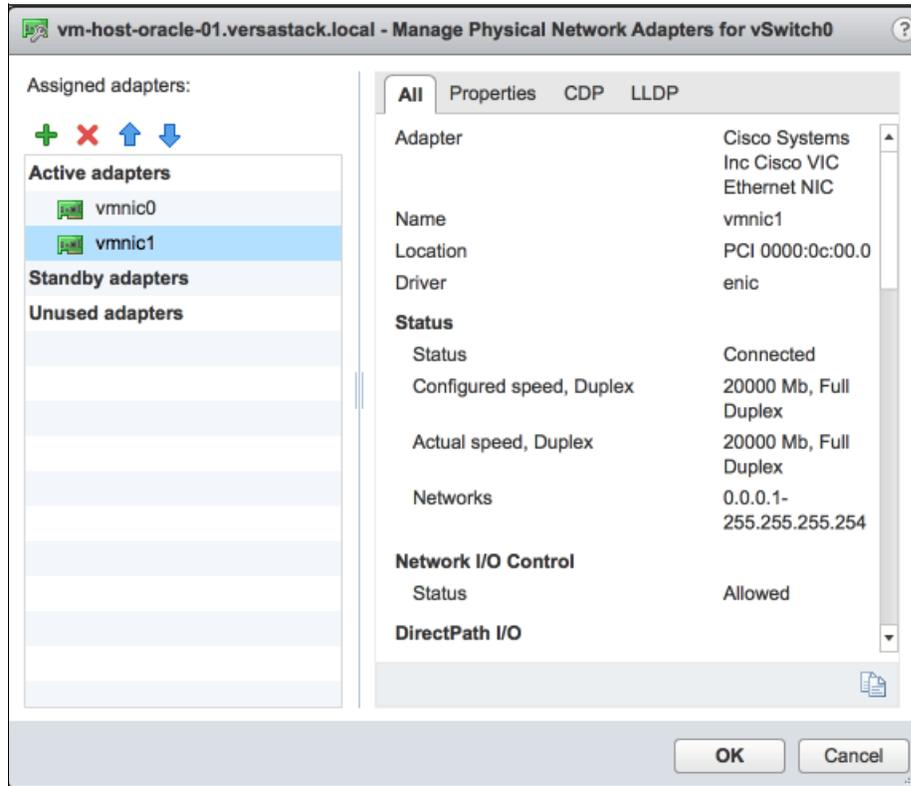
Figure 7-26 Manage physical network adapters for vSwitch0
