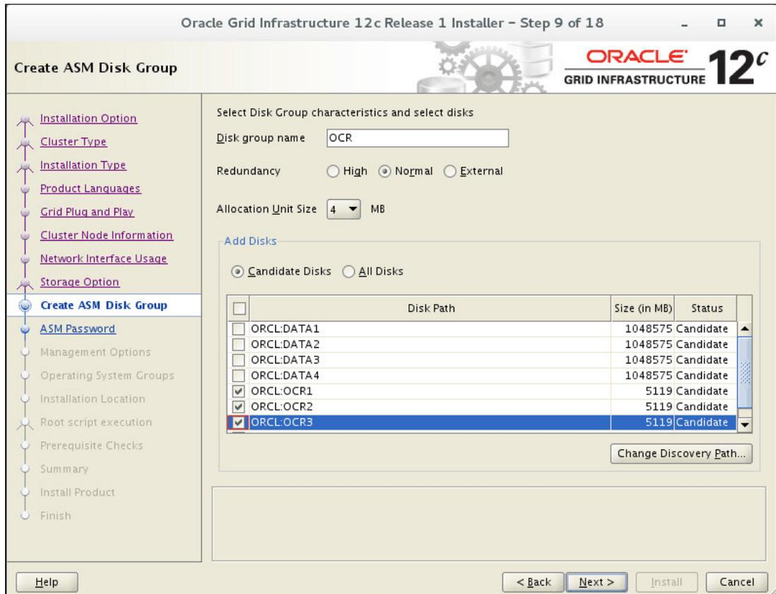
Figure 8-16 Create ASM disk group for OCR and voting disk files
