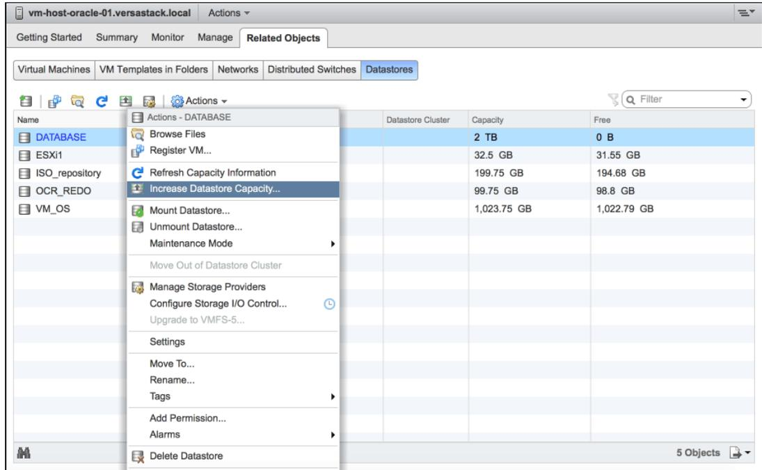
Figure 7-19 Increase Datastore Capacity
