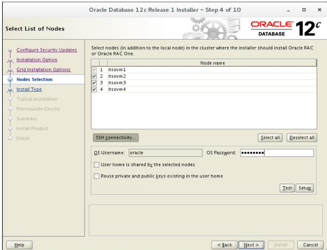
Figure 8-36 Config nodes and passwordless SSH connectivity for oracle user
