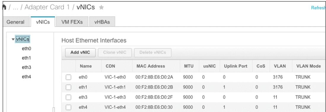
Figure 2-7 Adding vNIC's on Adapter 1
