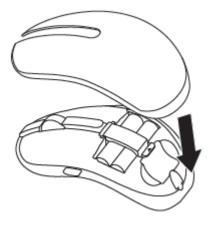
6 Slide the power switch to power on the mouse.
