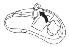
3 Install the AAA batteries into the battery compartment.
