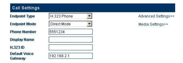
Under this mode, the GoIP operates in the point-to-point status. The setting parameters are as follows:
