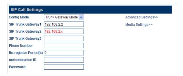
The trunk gateway is used to connect the VoIP network with the GSM network and convert the related protocols, so that users served by the two networks can call each other.
