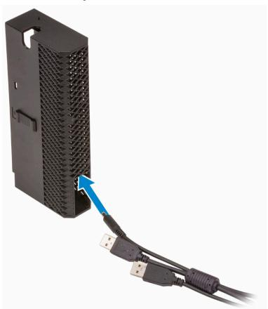
2 Connect the cables to their respective ports and turn the antenna (if available/applicable) outwards to pass through the antenna slot at the top of the cable cover.
