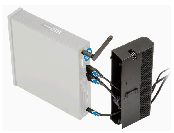
3 Align the cable cover retaining hooks into their slots on the Dell OptiPlex Micro chassis.
