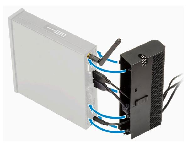
Gently press down on the cable cover (1) till it clicks into place and slide the latch (2) to lock the cable cover in place.
