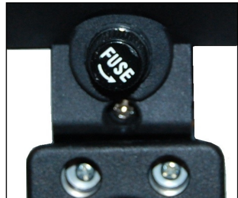
Figure 27: 3 AMP Tiller Fuse
