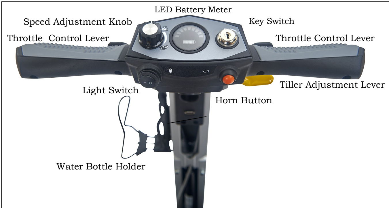
Figure 5. Carry On Tiller Control Panel
