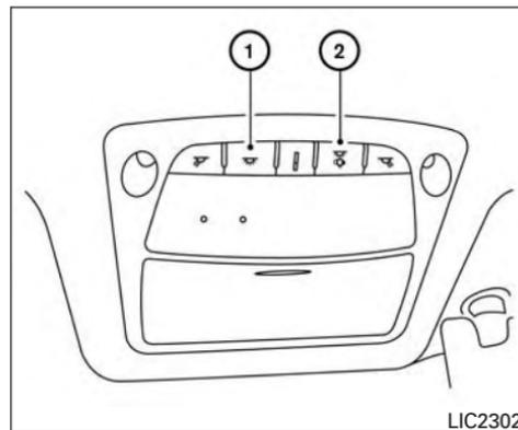
When the ON switch ① is pressed, the footwell lights (if so equipped), step lights (if so equipped), map lights and rear personal lights will automatically turn on and stay on for a period of time when:
