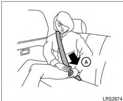
2. Slowly pull the seat belt out of the retractor and insert the tongue into the buckle (A) until you hear and feel the latch engage.
