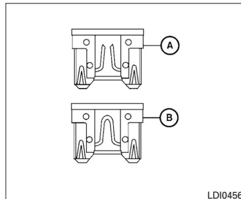
4. If the fuse is open (A), replace it with an equivalent good fuse (B).
