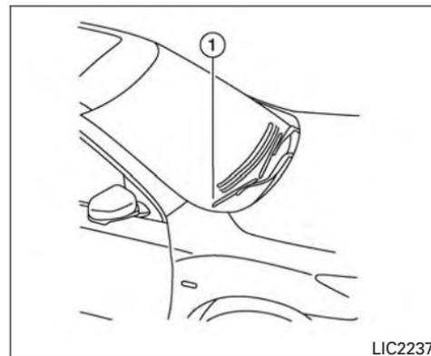
**Be sure you do not put anything on top of the autolight sensor located in the top side of the instrument panel ①. The autolight sensor controls the autolight; if it is covered, the autolight sensor reacts as if it is dark out and the headlights will illuminate. If this occurs while parked with the engine off and the ignition switch placed in the ON position, your vehicle’s battery could become discharged.**
