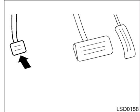
**To engage:** Firmly depress the parking brake.
