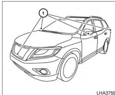
To display the multiple views, the Around View® Monitor system uses cameras located in the front grille, on the vehicle's outside mirrors and one just above the vehicle's license plate ①.
