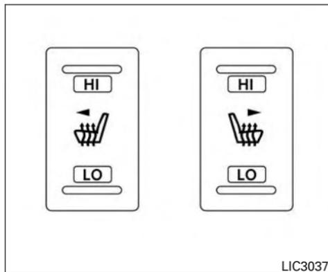
The 2nd row seats are warmed by built-in heaters. The switches are located on the rear of the front center console and can be operated independently of each other.
