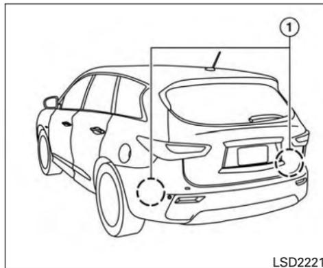
The BSW system uses radar sensors
