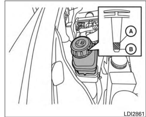
Check the fluid level in the reservoir.
