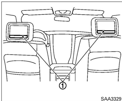
The rear displays are located on the back of the front head restraints (headrests).
