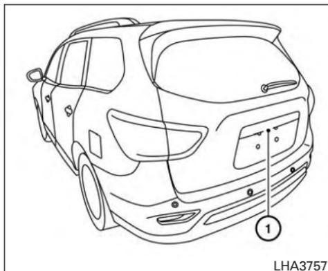
If dirt, rain or snow accumulates on the camera ①, the RearView Monitor may not display objects clearly. Clean the camera by wiping it with a cloth dampened with a diluted mild cleaning agent and then wiping it with a dry cloth.
