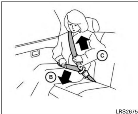
3. Position the lap belt portion **low and snug on the hips (B)** as shown.
