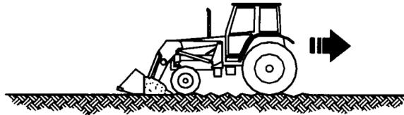
Backgrade work surface with a loaded bucket. Release all pressure on lift cylinders so full weight of bucket is scraping ground. Use heel of bucket
