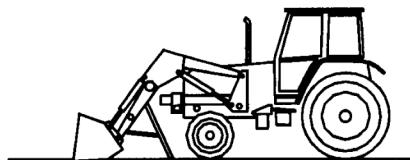
On self leveling loaders, the bucket will roll back at the same time the loader is lowered. Therefore, operate both hydraulic levers together.
