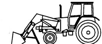
On some mountings, the lift cylinders must be extended more while the tractor is backing up, so that the subframes clear the front axle.
