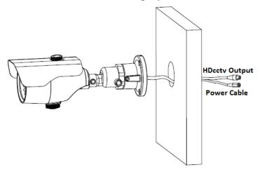
3. Screw the camera to the wall / ceiling.
