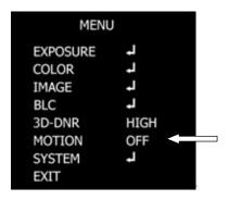
Switch to HIGH, MIDDLE, LOW and OFF to enable or disable noise reduction on dynamic recordings.
