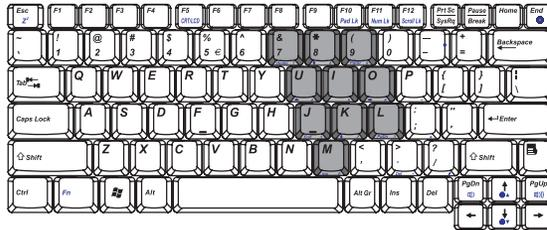
The embedded numeric keypad functions like a desktop numeric keypad. It is indicated by small characters located on the upper right corner of the keycaps.
