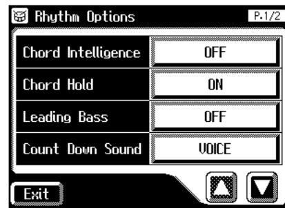
5. Touch the Chord Hold setting to switch between "ON" and "OFF."
