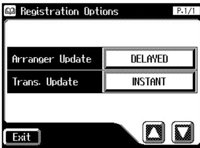
5. Touch the Arranger Update setting to switch between "DELAYED" and "INSTANT."
