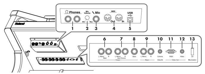
The functions of the jacks on the bottom of the keyboard are described below.
