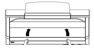
**1.** To open the lid, hold handles with both hands and lift it straight up. Then, slide it to the rear.
