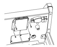
**1.** Connect the USB cable of the floppy disk drive to the ATELIER's Ext Drive connector.
