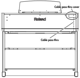
\* The side boards of the stand have grooves that allow the cables to be routed inside. You may use these if desired. For details, refer to the separate leaflet "STAND ASSEMBLY."
