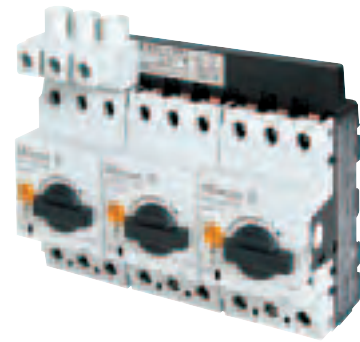
Photo 4: A PKZM0 motor protective starter grouping is linked on its supply side via a 3 phase bus connector bus. The motor protectors are fed using a common incoming terminal block BK25...-E , which features larger, distribution size electrical clearances to fulfill the requirements of a „Type E construction“.
