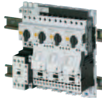
Photo 5: Examples of UL 508 Type F Combination Starters, which consist of UL 508 manual self-protected Type E Combination controllers combined with standard magnetic contactors.
