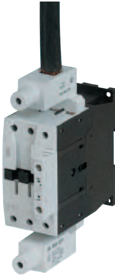
Photo 9: The paralleling bridge allows the AC-1 „General Purpose“ 3 phase current rating of the contactor to be increased by a factor 2.5 times its value. This accessory is especially useful when switching single phase resistive loads (such as heaters). It permits the use of smaller, and more economical, contactors to handle the load.
