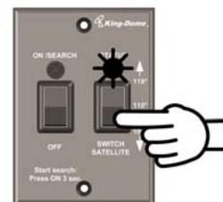
2. a) If you are locked onto the 119 satellite, press the hand held multi switch TO THE LEFT, or the wall mount multi-switch DOWN for one second.
