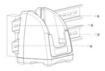
In either case, **after wall mounting,** it is **recommended** that the cables be secured to the DIN rail through use of a wire tie to prevent damage to the HomeBase/IntelliBase unit in case accidental or excessive force is applied to the cables.
