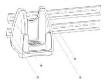
When using right-angle style RS-232 connector cable, the DIN rails may be mounted directly to the wall. When using standard RS-232 connector cables, it is recommended that the rails be mounted to the wall using a 25mm (1 in.) spacer to allow for appropriate strain relief of the cables.
