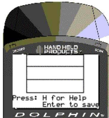
ALD mode searches for linear bar codes across the middle of the image. How much of the image is searched is controlled by the window size. This mode only works on linear symbologies and only decodes them horizontally. The following key presses configure this feature:
