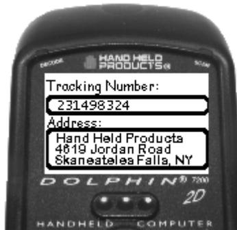
The data shown is information contained in the barcode. Press the <ENTER> key and the signature captured screen will be displayed as shown below:
