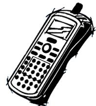
The **Dolphin® 7200 RS-232** terminal is identical to the Dolphin 7200 Batch terminal except that it features a micro-DB9 RS-232 port for serial data input/output and charging.
