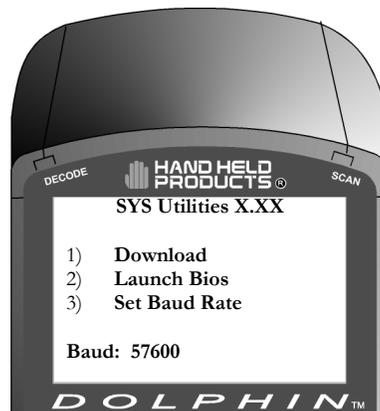
4. Press “3” to select Baud rate. Press “1” to set baud rate to 57600.
