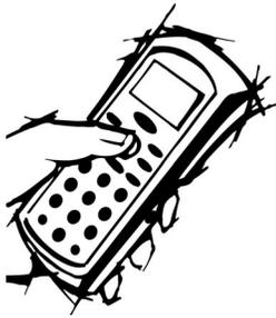
Dolphin is one of the most durable devices available, and is designed to withstand repeated five-foot drops onto a concrete floor. It also resists extreme temperatures, humidity levels and dust conditions.
