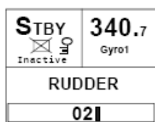
Inactive control unit
