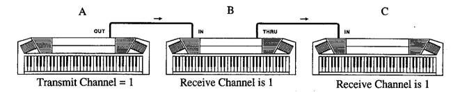
Next, in the arrangement shown below, if the receive channel for Instrument C only is changed to [2], with Instruments A and B on the same channel, you will then be able to control B with A, but because Instruments A and C are now on different channels, control is not possible. With channels in such an arrangement, it becomes necessary to set things up in order to control a designated instrument. With this keyboard, all channels can be used to receive signals.
