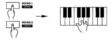
4. Press either the SOUND 1 or SOUND 2 button to turn off the Dual function.
