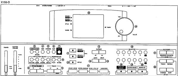
The buttons marked with a black dot ( • ) in the above illustrations have LEDs which light when the button is pressed. The buttons not marked with a black dot will not light when pressed.
