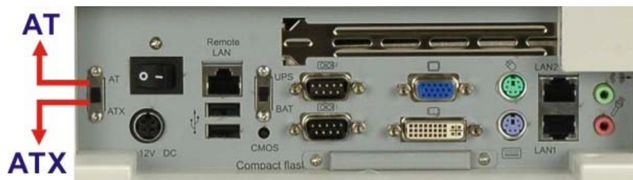
Figure 4-6: AT/ATX Switch Location
