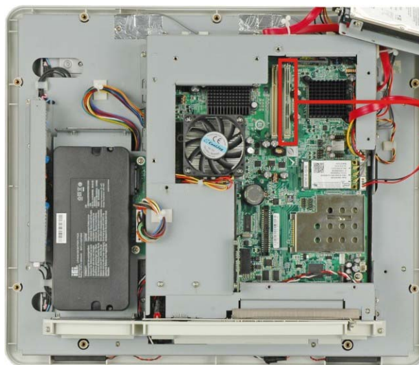
Figure 5-5: SO-DIMM Socket Locations
