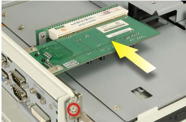
Figure 4-3: PCI Card Installation
