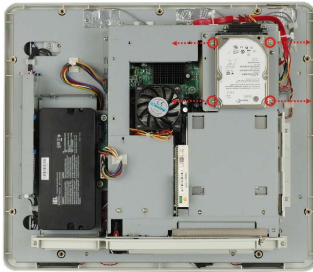
Figure 5-3: Hard Drive Retention Screws
