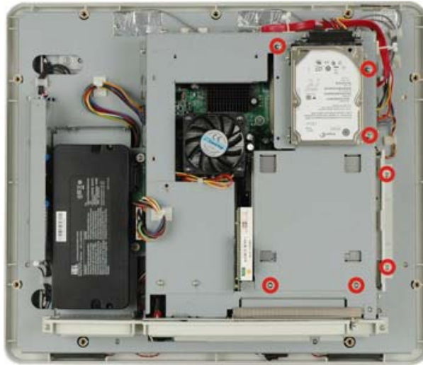
Figure 5-4: Platform Retention Screws
