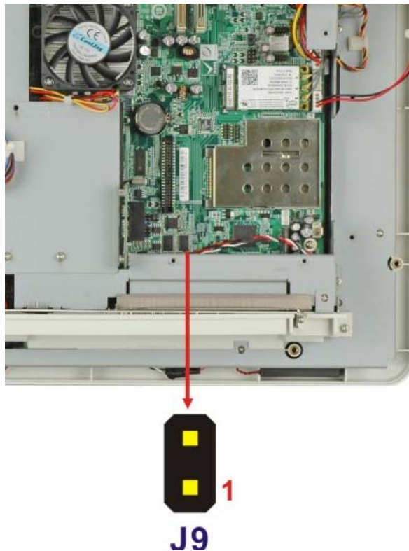
Figure 5-8: COM Port Voltage Select Jumper Location
