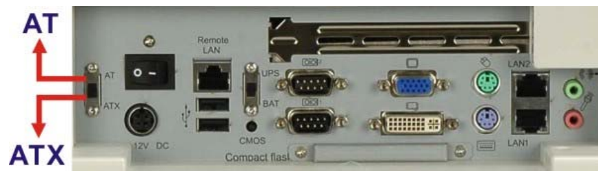
Figure 2-13: AT/ATX Mode Switch
