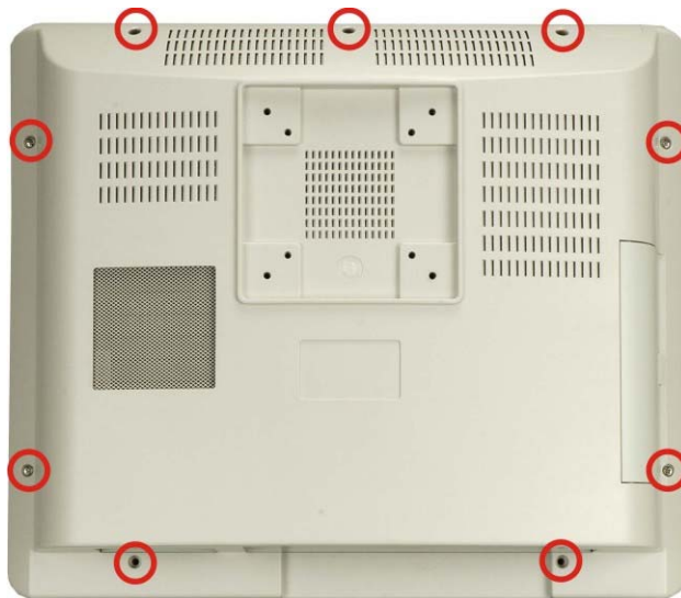
Figure 5-1: Back Cover Retention Screws
