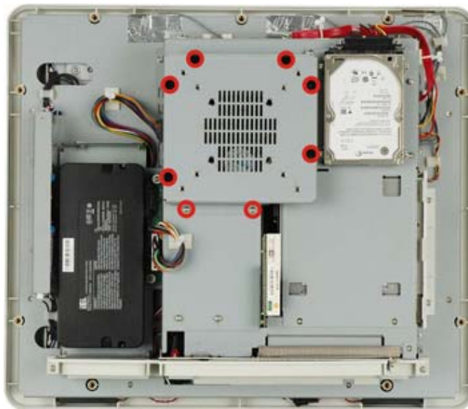
Figure 5-2: Wall Mount Bracket Retention Screws
