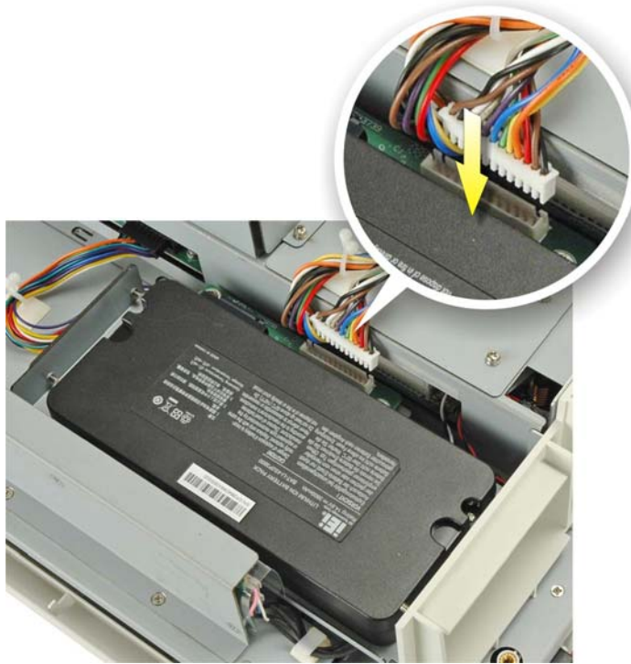
Figure 4-2: Connect the Battery
