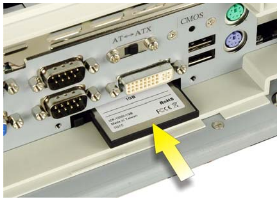
Figure 4-5: CF Card Installation
