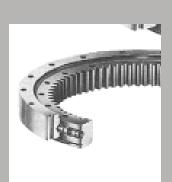
Slewing Rim Bearings are designed to carry both axial and radial loading in addition to being able to handle moment and overturning loading. These bearings are used in applications for support of large rotating and pivoting units used in construction equipment such as power shovels, track cranes and loaders. They are also popular in applications like machine tool tables and wind turbines.
