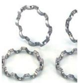
**CAGE FORMING** – The cages go through several press forming operations before they are in their finished shape. If rivets are to be used they are then punched with rivet holes.
