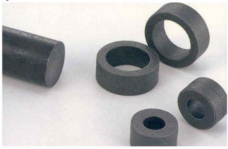
**RING TURNING** – The forged rings are then sent to CNC turning centers or multi-spindle chuckers to be turned and machined into the required part shape.
