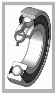
The cages of rolling element bearings must be able maintain proper spacing of the rolling elements, have the strength to withstand centrifugal and shock forces and be able to tolerate temperature and lubricant variations.
