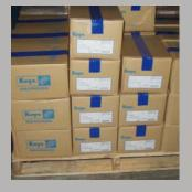
DO store bearings on a pallet, which is definitely a better choice than directly on the floor with no protection from moisture and vibrations from machinery.
